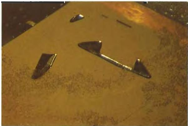
Figure 14. This large metallic inclusion, accompanied by numerous pinpoint inclusions, was seen beneath the table facet of HPHT-treated sample 21475 (see also figure 5). Note the rectangular area marked by graining; the border of this rectangular area is outlined by sectors that luminesce green to visible light. Photomicrograph by John I. Koivula; magnified 35 $\times$ .
