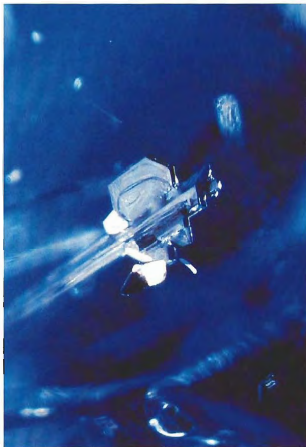
Figure 12. The shiny metallic appearance of platinum is very evident in this large, thick, angular platinum inclusion in a Chatham flux-grown synthetic blue sapphire. Magnified 35 \times .
