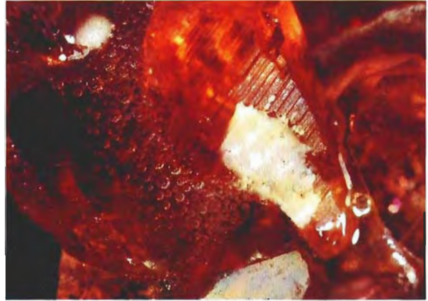
Figure 2. Dense concentration of spherical gas bubbles in the silica-based ceramic glaze applied to the back of this Chatham flux-grown synthetic orange sapphire crystal group. Oblique illumination accentuates the termination of the glaze near the edge of the crystal group. Magnified 10×.
