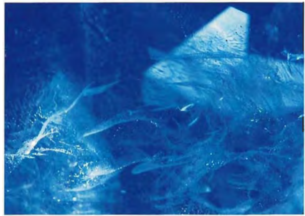
Figure 9. White, wispy veils of flux, fine in texture, betray the synthetic origin of this Chatham flux-grown blue sapphire. Note the thin, white-appearing needle in the upper left of this photomicrograph. Magnified 15 \times .
