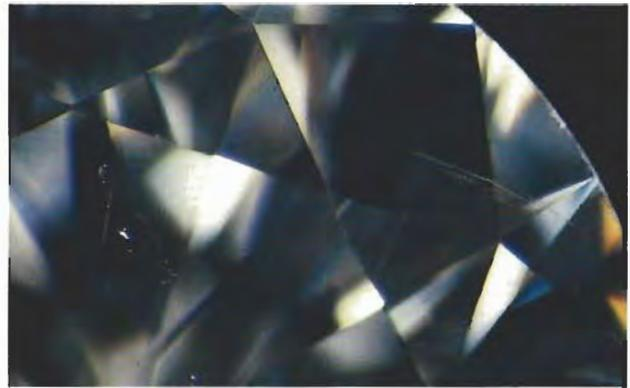
Figure 4. The small cleavages shown here contributed to the  $SI_1$  clarity grade in this 0.51-ct diamond (no. 4 in table 1) before treatment (left). After treatment (right), the clarity was graded as  $VS_2$ . Magnified  $15\times$ .
