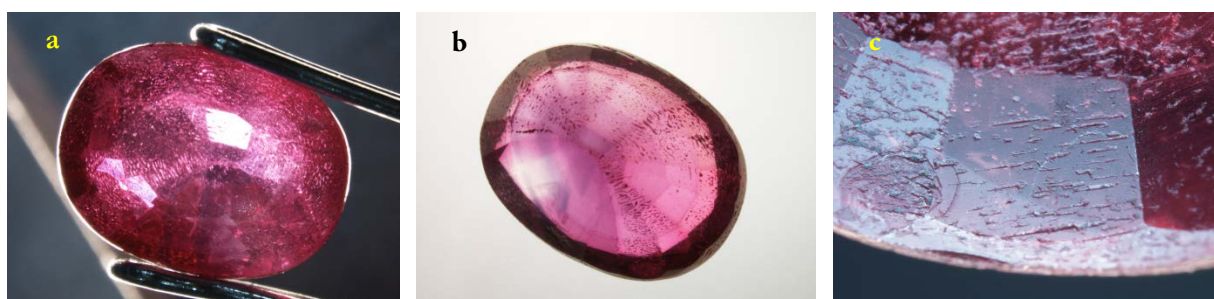
Figure 5: Sample 389 taken under a) dark field illumination and b) diffuse light illumination, magnified 7.5x; c) flux inclusions reaching to the surface, magnified 35x can be seen in all seven samples on the synthetic ruby overgrowth of type II samples. Photo by J. Muiyal © GIA
