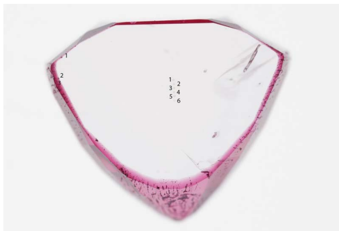
Figure 8: Wafer of GLA reference sample 391 showing the location of the laser spots in synthetic ruby at the edge and natural seed at the center. The photo was color calibrated and captured using transmitted light. Photo: S. Engniwat © GLA.
