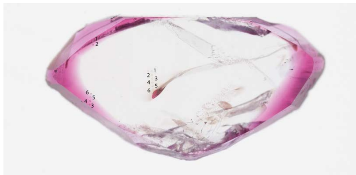
Figure 7: Wafer of GLA reference sample 385 showing the location of the laser spots in synthetic ruby at the edge and natural seed at the center. The photo was color calibrated and captured using transmitted light. Photo: S. Engniwat © GLA.
