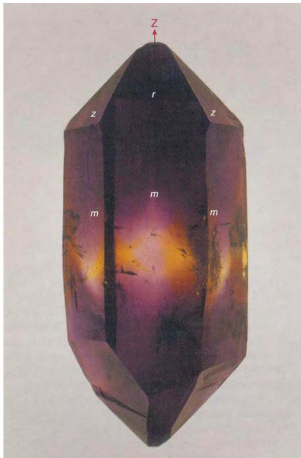
Figure 7. Prismatic crystals of synthetic amethyst are grown in alkaline solutions on seeds that are nearly cubic in shape. Such crystals have well-developed  $m$ ,  $r$ , and  $z$  faces, and their morphology closely resembles that of natural quartz crystals. The yellow color in the center of the prism correlates to  $c$  sectors, whereas the amethyst areas consist of rhombohedral sectors. Photos by V. S. Balitsky.
