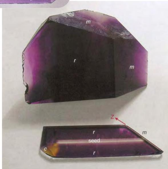
Figure 5. Synthetic amethyst crystals grown in alkaline  $K_2CO_3$  solutions on seed plates cut parallel to  $r$  are dominated by  $r$  sectors. The 2-mm-thick plate on the bottom was sliced parallel to  $a$  from a similar crystal. The inset shows numerous polysynthetic Brazil twins in the  $r$  sector, which were brought out by etching the slab in a strong  $NH_4F \cdot HF$  solution. Photos by V. S. Balitsky.
