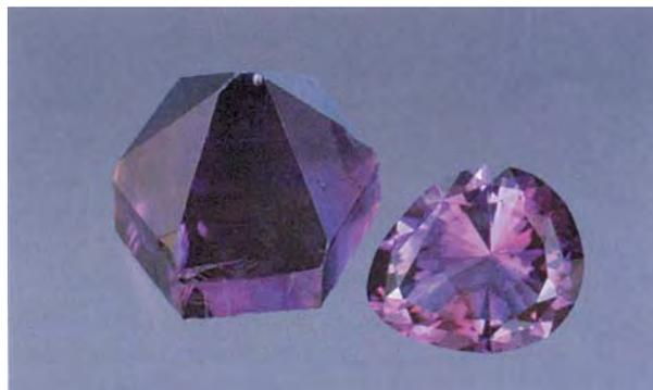
Figure 8. The ends of the prismatic crystals can be faceted to yield high-quality synthetic amethyst, which will consist of both  $z$  and  $r$  sectors. The crystal termination measures 2.4 cm high. Photo by Maha Tannous.
