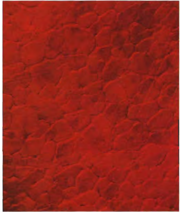
Figure 4. The "honeycomb" structure shown by pinfire "Opalite" when examined with shadowed transmitted light is characteristic of a laboratory-grown material. Magnified 15×.
