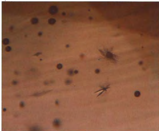
Figure 7. Bubbles and devitrification crystals help identify this sample as a purple Ca-phosphate glass. Immersion, magnified 35 \times .
