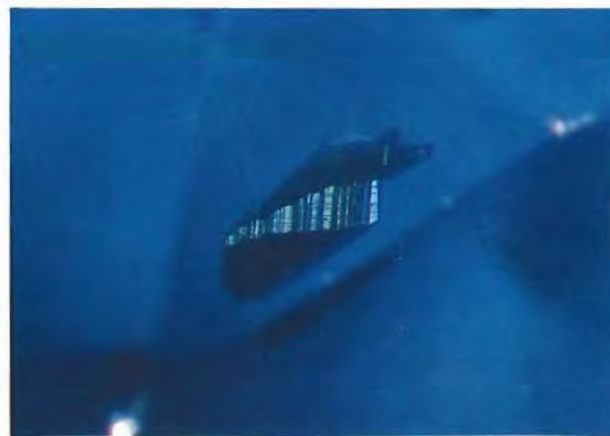
Figure 24. Opaque, black crystals of ilmenite—observed in different euhedral to subhedral forms—were another addition to the diverse mineral inclusions found in the southern Vietnam sapphires. Oblique fiber-optic illumination, magnified 35 \times .
