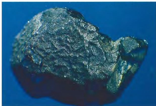
Figure 8. The rough crystal surfaces of the southern Vietnam sapphires displayed the heavy dissolution effects typical of corundums that have been brought to the surface by alkali basalts. Overhead illumination.
