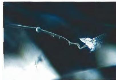
drill hole is an earmark of early laser technology, which was first noted in *Gems & Gemology* in the Fall 1970 issue (p. 224). Refinements in the laser-drilling process over the next few years led to laser drill holes without this cone-shaped point of entry.
