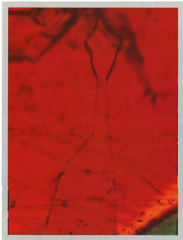
Figure 15. Structural characteristics are not always easy to recognize. Note this "distorted" umbrella pattern found in a faceted Douros synthetic ruby. These peculiar growth structures, with r, d, and r' sectors, were observed in immersion at 50× magnification.
