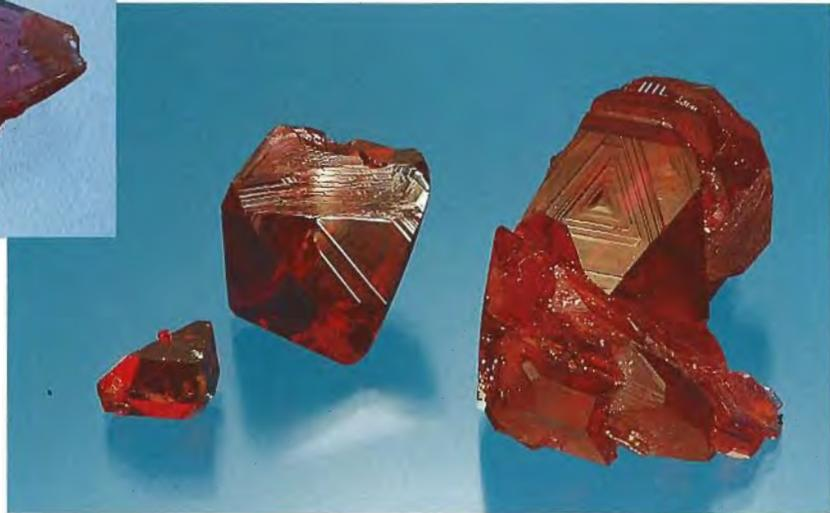
two new surfaces produced when an irregular intergrowth of two rhombohedral crystals (samples D1 and D2) of random mutual orientation was sawn and polished. For the microscopic examination of one of the tabular crystals (to obtain a cross-section between the two basal pinacoids), we had a slice cut perpendicular to the basal pinacoid *c*. Three microprobe scans of 50 point analyses each were performed on this 2.2-mm-thick polished slab on the surface at the cross-section.
