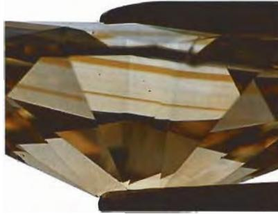
*Figure 6. Parallel color banding is sharply defined in this 1.08-ct marquise brilliant-cut diamond, which measures 10.71 × 5.25 × 3.26 mm. Magnified 17×.*
