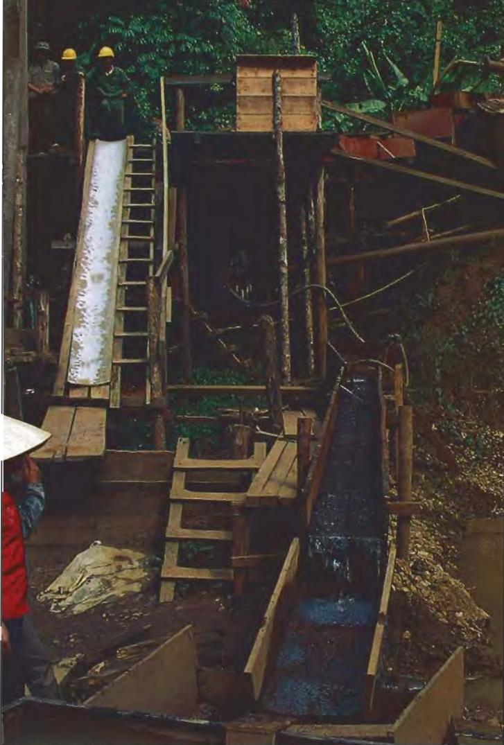
Figure 3. From the pit shown in figure 2, the gem-bearing gravels were pumped to this large sluicing system that, at the time (November 1992), was about 30 m away. The heavy-mineral concentrate collected here, at the end of the system, was then taken to the mine headquarters. Photo by Robert C. Kammerling.
