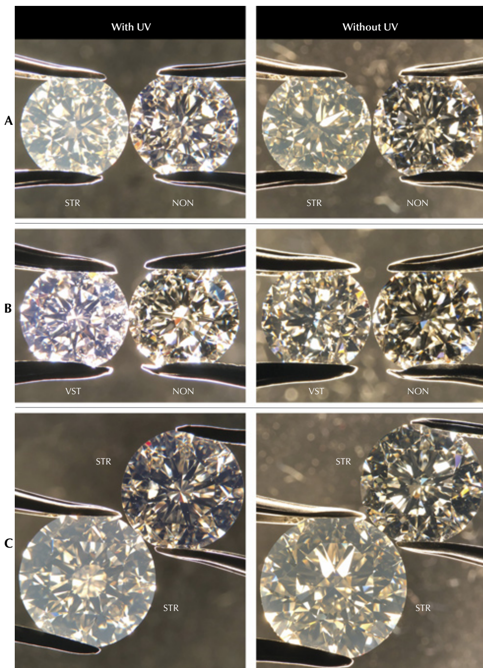
Figure 10. Sets of diamonds with different UV intensities were examined and imaged under microscope darkfield illumination, with and without UV content.
