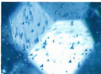
Figure 18. Several synthetic sapphires mixed with natural sapphires in an Art Deco-style pin contained unusual, and possibly confusing, triangular inclusions that contain bubbles. Magnified 30 \times .
