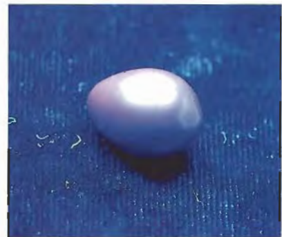
Figure 9. The pink-to-red fluorescence to long-wave U.V. radiation proves natural color in the pearl shown in figure 8.
