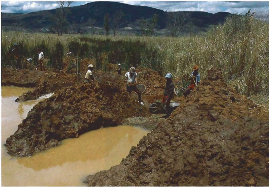
Figure 14. Washing ponds were created downhill from the main excavation site at Ouro Fino to separate the small pieces of tourmaline from the hardened soil in which they had been encased.
