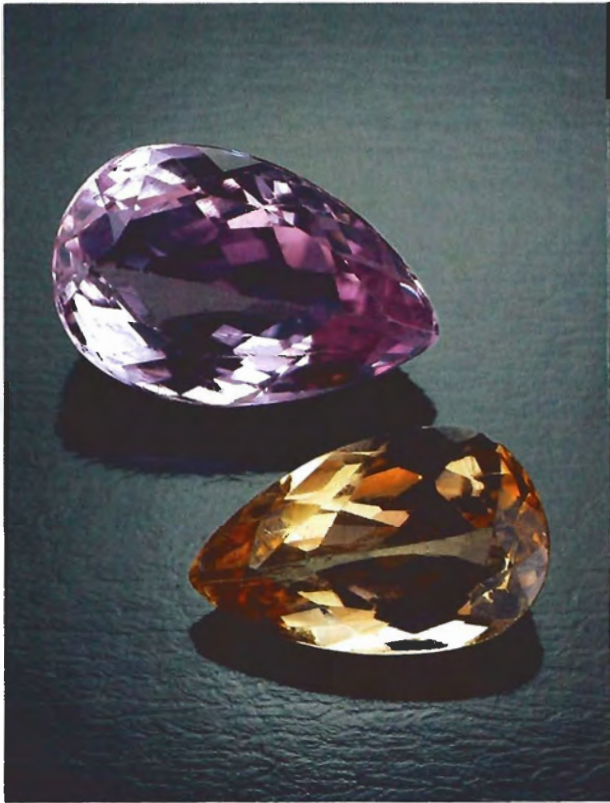
Figure 7. Heat treatment over an open flame turned a yellow topaz from the same lot as the 2.5-ct stone on the lower right into the attractive pink topaz on the upper left. Stones courtesy of P. Flusser, Overland Gems, Los Angeles, CA; photo © Tino Hammid.
