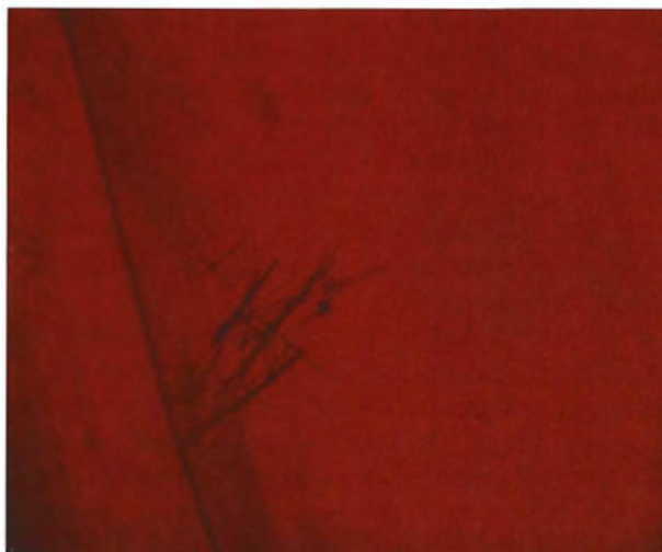
Figure 4. A small group of extremely fine acicular inclusions found in the crystal shown in figure 1. Transmitted light, magnified 50 \times .
