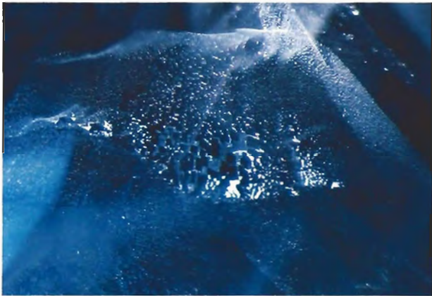
Figure 4. Flux ranging from semitransparent to opaque and from near-colorless to white occurs in wide, mesh-like patterns intersected by thin, tightly arranged white "fingerprints" in a Lechleitner synthetic blue sapphire. Dark-field illumination, magnified 35 \times .
