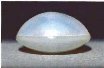
Figure 6. Profile of a Mabe pearl showing nacre shell cemented to a mother-of-pearl base.
