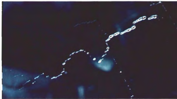
Figure 5. "Internal lightning," caused by an internal electrical discharge during irradiation in a linear accelerator, is evident when this 52.3-ct blue topaz is viewed through the table with the unaided eye (left) as well as with 3× magnification (above). Stone courtesy of P. Flusser, Overland Gems, Los Angeles, CA; photos © Tino Hammid.
