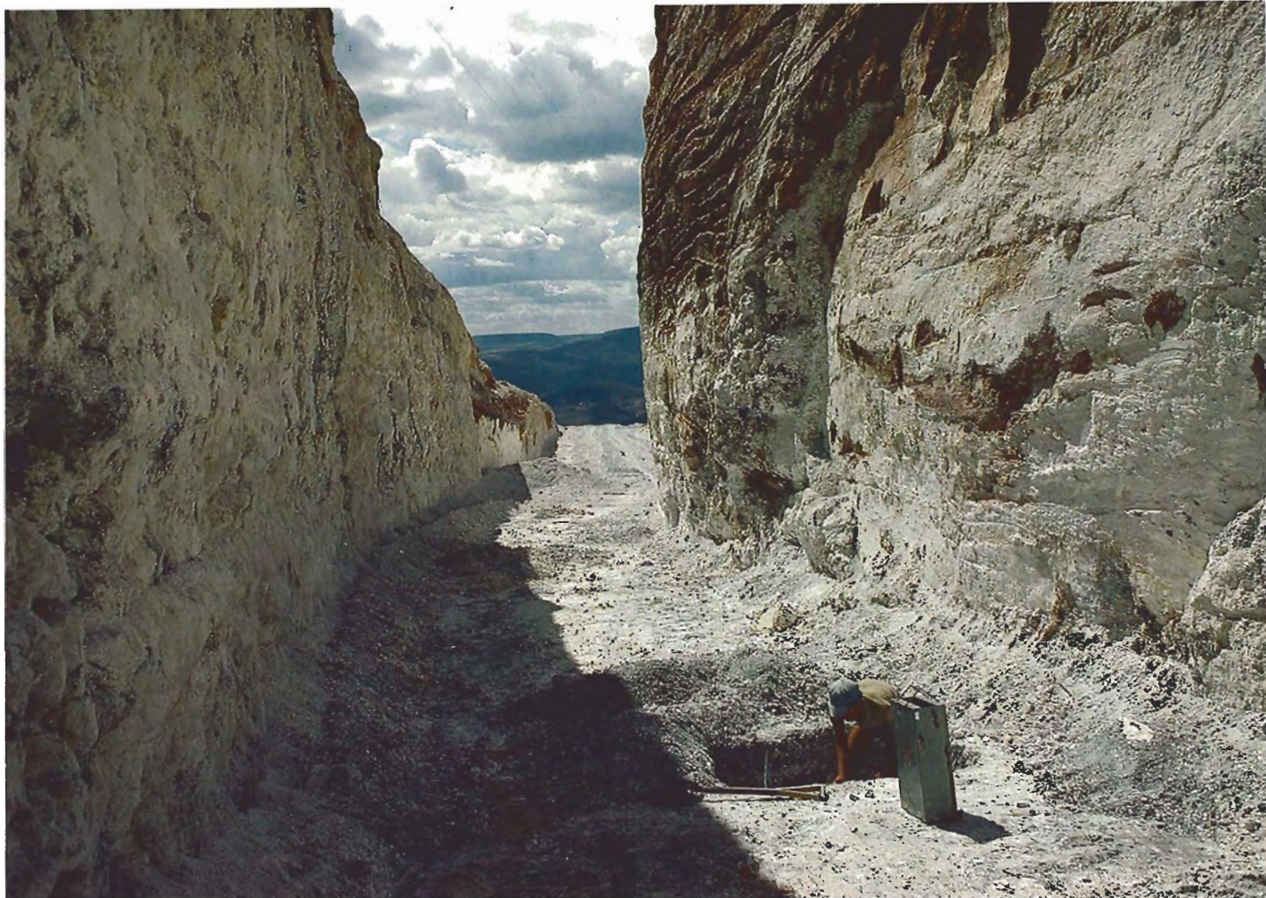
Figure 9. More than 30 years of bulldozing through the pegmatite at the Salinas mine has produced a "canyon" that is 30 m deep in some areas. Here a garimpeiro works a "pocket" where gem material was spotted when the bulldozer made its most recent pass. The box on the side of his diggings was provided by the mine owner to safeguard any crystals found. On the right wall, the sharp contact between the kaolin of the pegmatite and the red lateritic soil that covers it is evident.
