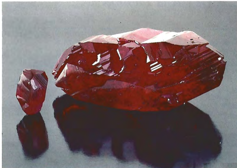
Figure 5. Synthetic ruby crystals grown by Chatham, Inc., using a technique by which Verneuil synthetic rubies are placed in a flux-growth environment. Like the Lechleitner synthetics, these crystals contain both curved striae and flux. Photo on left ©Tino Hammid; photomicrograph, dark-field illumination, magnified 40 \times .
