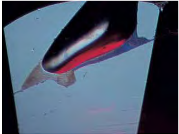
Figure 16. One example recently submitted to the GIA Laboratory showed an obvious oxidation of the glass at the surface. Photomicrograph by S. F. McClure; magnified 40 \times .
