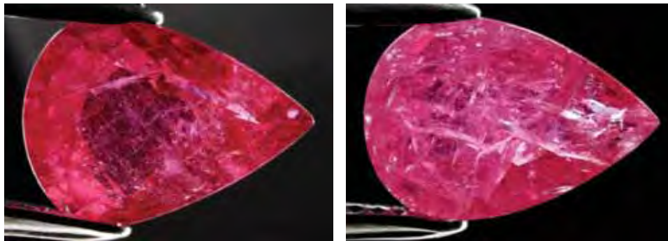
Figure 24. Caustic soda was used to see how much damage a stronger base solution would inflict on the glass. The image on the left shows the 2.08 ct lead glass-filled ruby before the test began; after one hour of exposure (right), the damage to the filler was significant. Photomicrographs by C. P. Smith.
