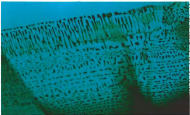
Figure 8. Typical secondary "fingerprint" in one of the faceted Russian flux-grown synthetic emeralds. Partial polarized light, magnified 45x.
