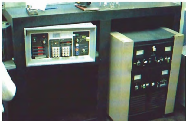
Figure 1. The laser saw unit consists of a large cabinet that houses the power amplifier for the flash lamps (on the right), a smaller cabinet that encloses the laser rod (center), and an x-y platform computer (off to the left).
