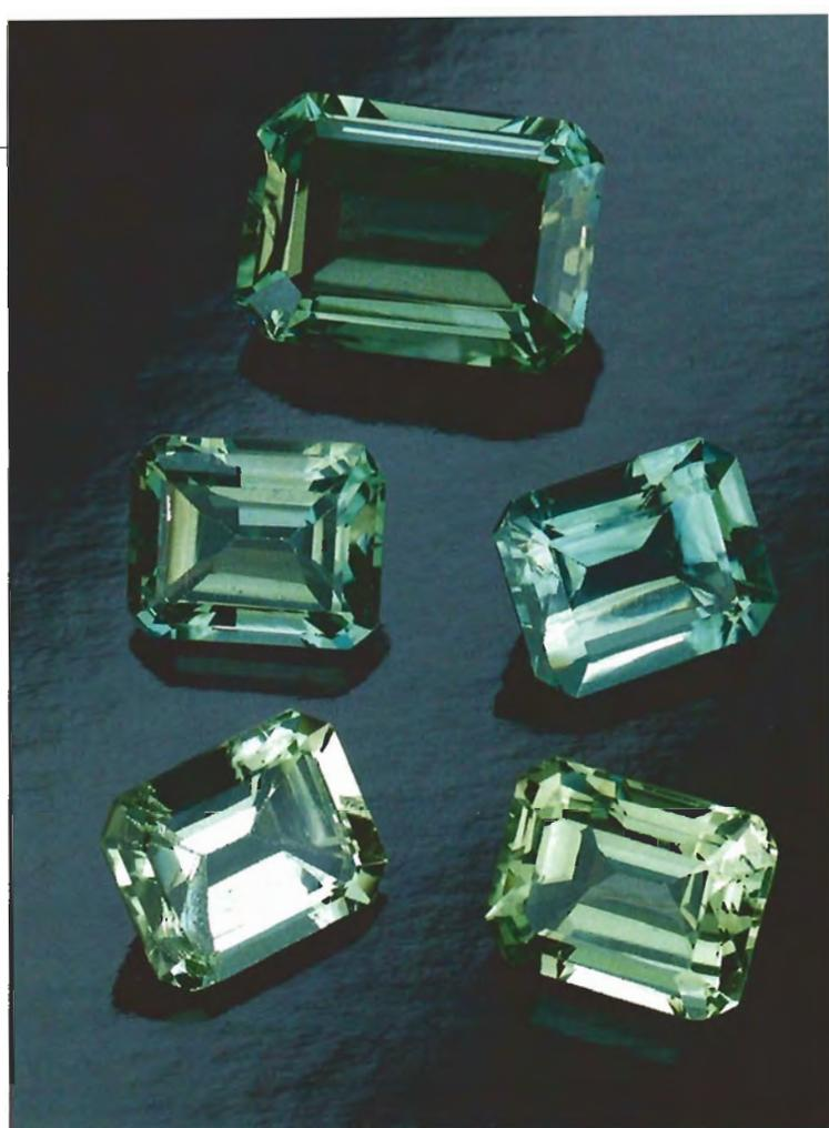
Figure 1. A new color variety of irradiated topaz has appeared in the trade, and is being sold under the name Ocean-green topaz. These samples (3.85–8.70 ct) show a typical range of color for this material. Photo © GIA and Tino Hammid.
