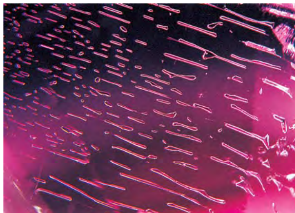
Figure 2. A healed fissure that traverses one side of this extraordinary gemstone consists of equidimensional-to-oblong liquid and liquid-gas inclusions in a parallel formation. Photomicrograph by C. P. Smith; magnified 28 \times .
