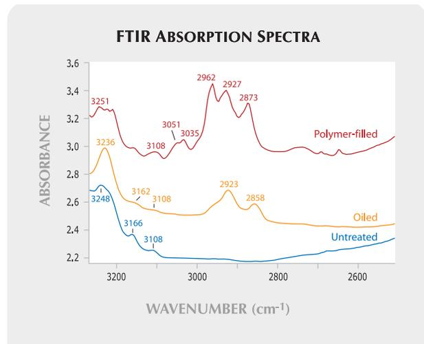
Figure 5. This representative mid-IR spectrum of the polymer-filled beads shows distinct features from polymer impregnation, particularly between 3100 and 2850  $\text{cm}^{-1}$ , that are not seen in the oiled and untreated aquamarine comparison samples. The absorption features at 3051 and 3035  $\text{cm}^{-1}$  are due to the benzene C-H bond in a polymer. The bands from 3250 to 3100  $\text{cm}^{-1}$  are characteristic of beryl. Spectra are offset and shifted vertically for clarity.
