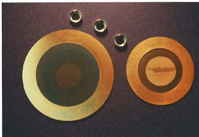
Figure 2. By the end of the 1980s, free-standing transparent, near-colorless synthetic diamond thin films as large as 2 cm ( 3/4 in.) in diameter were being grown by the new low-pressure technology. Such thin films are now used in masks for X-ray lithography (bottom) or as windows for X-ray fluorescence spectrometers (top). Photo courtesy of Crystallume.
