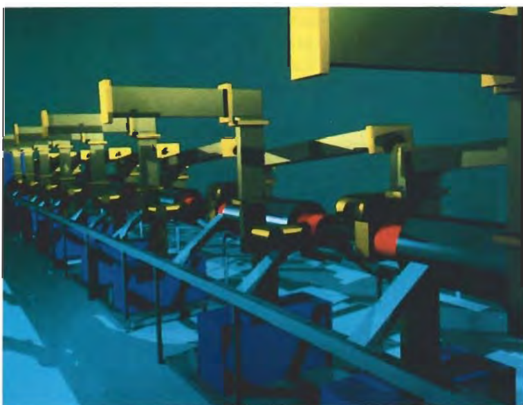
Figure 4. During the 1980s, great quantities of gem materials were irradiated in an electron accelerator for the purpose of inducing or enhancing color. This computer-generated image is the electron accelerator at the Rensselaer Polytechnic Institute, Troy, New York. Photo courtesy of Rensselaer Polytechnic Institute.
