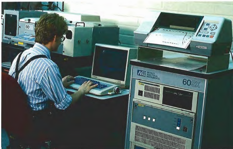
Figure 5. Although not a new technology, infrared spectroscopy has recently provided solutions to many tough gemological problems. The GIA Research Department has used this Nicolet 60SX FTIR spectrometer to identify treated materials such as irradiated diamonds and plastic-impregnated turquoise, as well as to separate some natural from synthetic emeralds, diamonds, and alexandrites. Photo by Robert Weldon.
