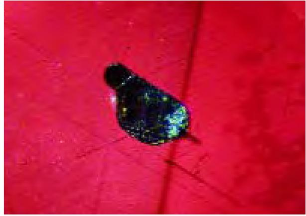
Figure 7. As with the Bekily garnets examined earlier, some of the Tranoroa pyrope-spessartines also contained tabular graphite crystals. Photomicrograph by L. Kiefert; magnified 100 $\times$ .
