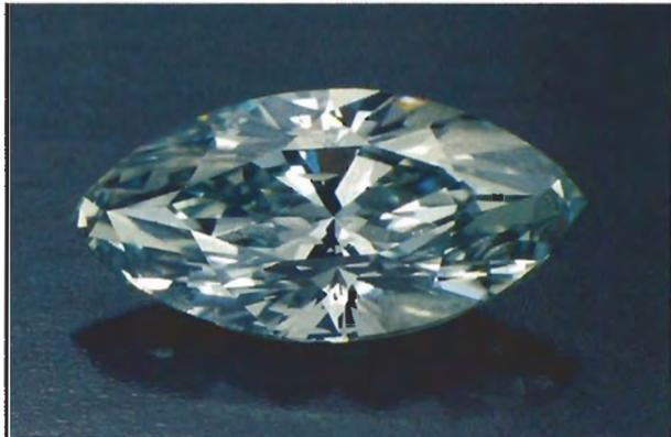
Figure 3. Stone E in this study is a natural-color gray non-electrically conductive type Ia diamond from the Argyle mine, in northwestern Australia. Stone courtesy of Argyle Diamonds; photo by Robert Weldon.
