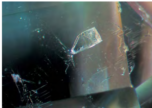
Figure 15. This inclusion in a Mt. Mica tourmaline was identified as feldspar by Raman analysis. Fluid inclusions also are visible in the immediate vicinity. Photomicrograph by John I. Koivula; magnified 20 \times .
