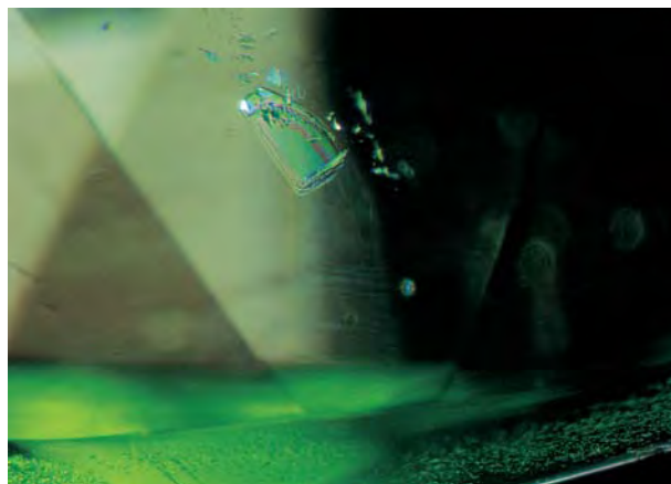
Figure 16. Cross-polarized light has produced interference colors in this inclusion, which is probably a crystal of tourmaline within tourmaline from Mt. Mica. Photomicrograph by John I. Koivula; magnified 15 \times .
