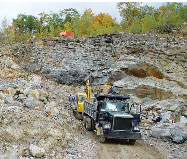
Figure 7. An excavator and dump truck are used to remove mined material from the open cut at Mt. Mica, as shown in this October 2004 photo by Gary Freeman.
