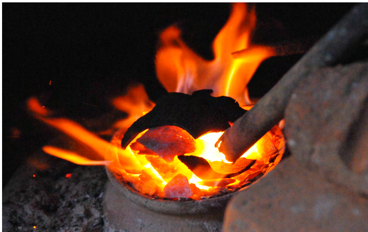
Figure 1: A ruby is heated at “low temperature” in air using the traditional blow pipe technique in Ratnapura (Sri Lanka). Photo: V. Pardieu © GIA
