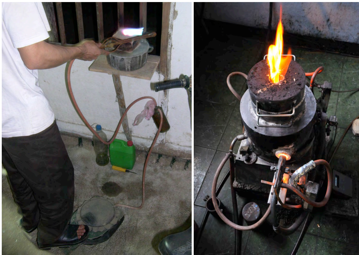
Figure 3: Left: A burner heating some rubies with a jeweler torch (snake bite technique) seen in Vietnam (2005). Right: One of the Lakmini furnaces, developed in the 1980's, and commonly used in Sri Lanka to heat blue sapphires. Photos: V. Pardieu
