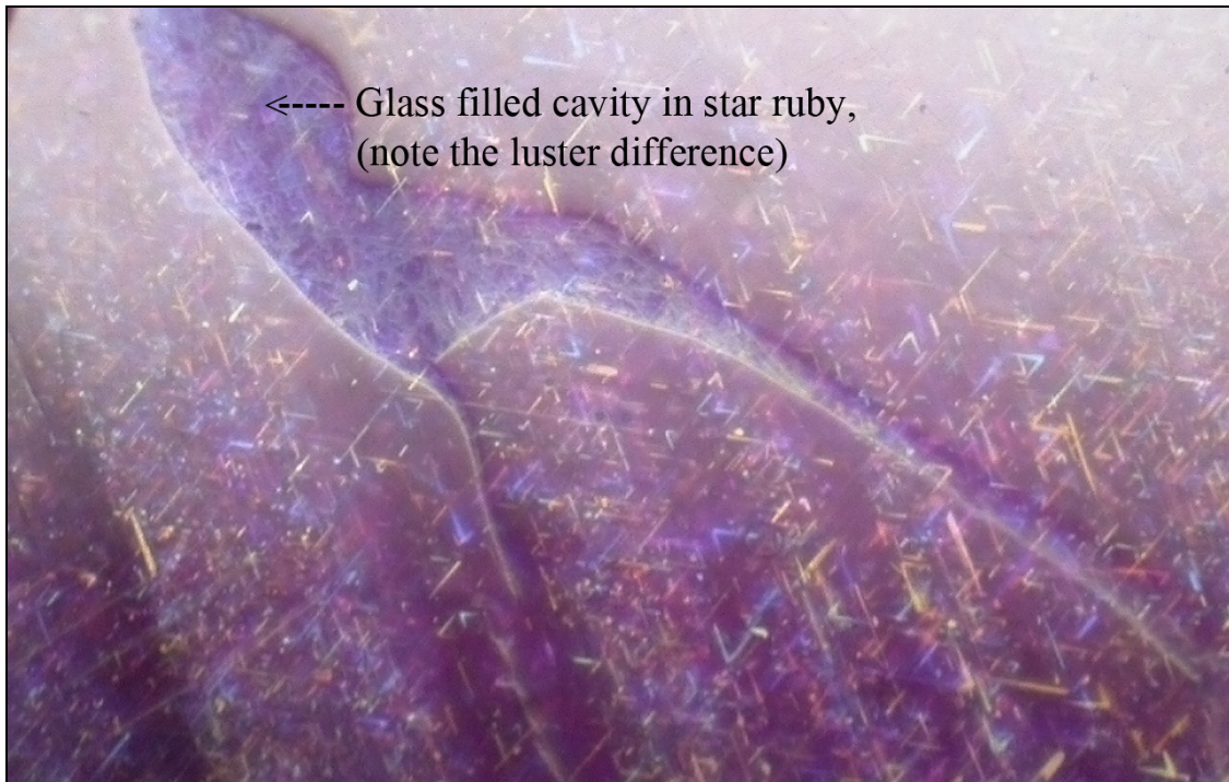
Figure 4: A glass filled cavity in a star ruby studied using overhead lighting. The numerous rutile needles were not affected by the glass filling process as the glass melting point is lower than the temperature necessary to affect them. Photo: V. Pardieu / AIGS, 2006
