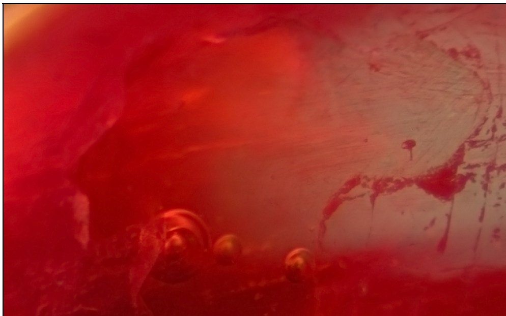
Figure 13: The identification of large glass filled cavities can also be challenging as the lead glass' refractive index is very close to the host's refractive index and the difference in luster is not obvious as shown here. Nevertheless in this example large gas bubbles are useful evidence to properly identify the presence of the glass filled cavity. However, this sample also shows that polishing has damaged some areas where the glass meets the ruby. Photo: V. Pardieu
