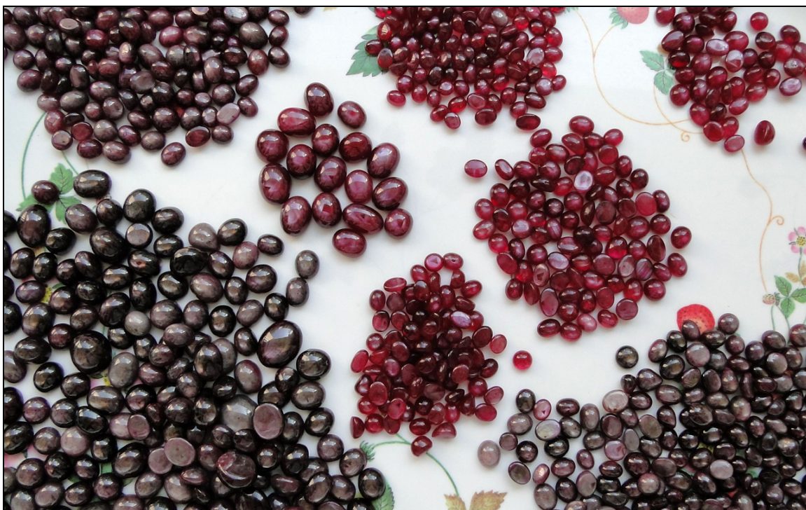
Figure 6: Several small parcels of lead glass filled rubies showing the different qualities produced by this treatment using as base ruby rough material reportedly from a single (still undisclosed) area in Madagascar. The stars are not visible here as the sky was cloudy; nevertheless the colors are representative of the stones seen at the burner's office. Photo: V. Pardieu, GIA Laboratory Bangkok, January 2010.
