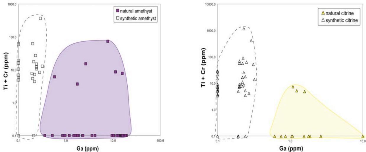
Figure 2. Chemistry plots for amethyst and citrine showing elevated Ga in natural stones and some Ti + Cr enrichment in synthetic samples. Note that the axes are log scale. (0.1 ppm was added to all plotted concentrations to facilitate log plotting of BDL results. Thus, a data point at 0.1 ppm represents a BDL result.)
