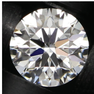
Fig. 1: Image taken in Carlsbad using the new L-Box for one of GIA's research diamonds. Note that the dark and light areas of the reflection pattern are very similar to the pattern seen by the typical observer in a diffused lighting environment. The L-Box environment creates a good replication of how a diamond is viewed in real life.
