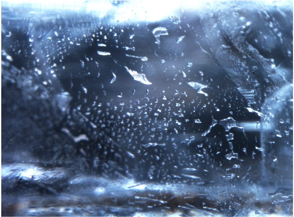
Figure 13: A fingerprint showing the fluid channels within its form in jeremejevite. Magnified 64x. Photo ©GIA.
