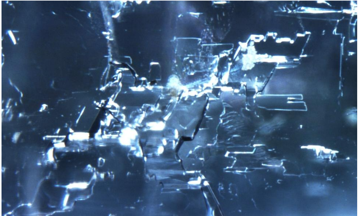
Figure 15: Fluid inclusions producing an interesting pattern in jeremejevite. Magnified 60x. Photo ©GIA.
