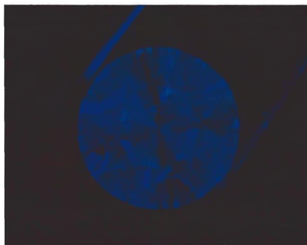
Figure 6. The cruciform fluorescence pattern as observed in the synthetic blue round brilliant when exposed to short-wave ultraviolet radiation. Magnified 6×.
