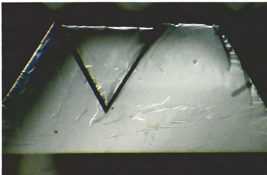
Figure 16. A single large trigon aids in the identification of this octahedral face on the largest rough synthetic diamond crystal. Oblique illumination and shadowing, magnified 50 \times .
