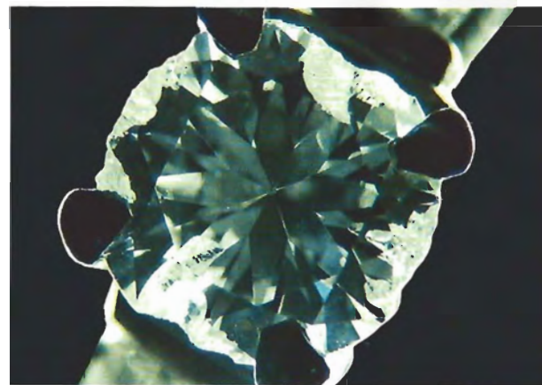
Figure 8. Even with diamond, the girdle can be severely damaged if it is not adequately protected.
