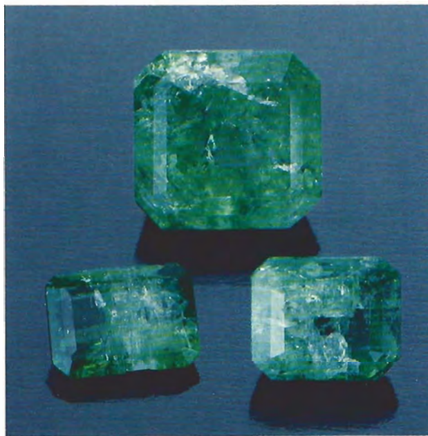
Figure 17. Most emeralds in the trade today are oiled (left). Their appearance may be altered radically (right) when the oil is driven out of the fractures by a procedure such as cleaning in an ultrasonic. Photos © Tino Hammid.
