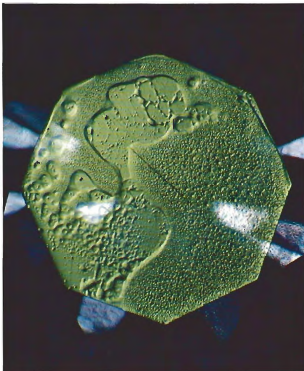
Figure 13. The use of a borax-containing soldering flux resulted in severe etching of the table of this sapphire. Photo by Robert E. Kane.
