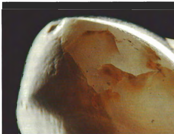
Figure 18. This star sapphire was stained when dirt was forced into the fractures during steam cleaning.
