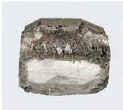
Figure 8. In this 0.87 ct sample (no. 49806a), shown here from two different views, near-colorless CVD synthetic diamond has been grown over a CVD substrate, resulting in a much thicker crystal than would have been produced with an HPHT synthetic diamond substrate. Note the precipitation of graphite and non-diamond carbon around the crystal that gives rise to the dark gray to black rim. Photos by Elizabeth Schrader.
