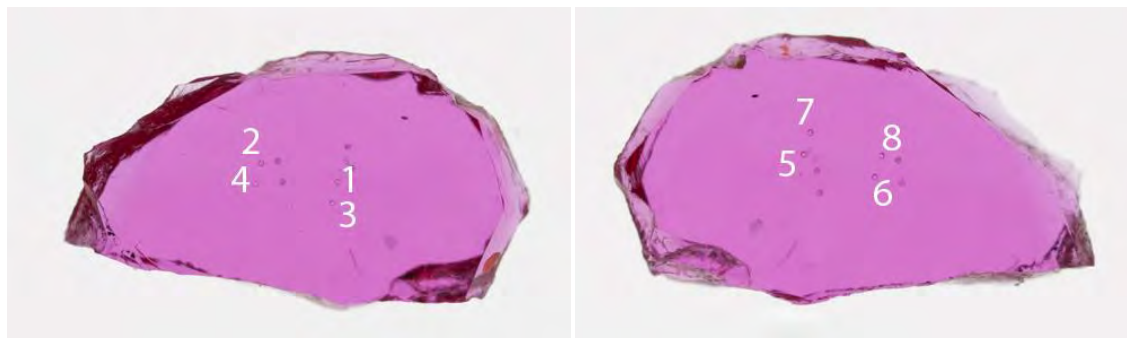
Figure 36: Two views of GIA reference sample 100305163897 (A2 type; see Annex C for a description of the classification system), seen after fabrication, showing the positions of the eight LA-ICP-MS spots. Photos (color calibrated): Sasithorn Engniwat © GIA.
