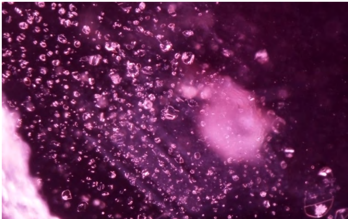
Figure 80: The same “A” type sample shown in the previous photo only focused slightly above the mica crystal to reveal a plane of numerous thin negative crystals/thin films. GIA reference sample 100305163925, an A type sample collected in the “Central” area in September 2012. Darkfield + fiber optic illumination, magnified 80x. Photo: Jonathan Muiyal © GIA.
