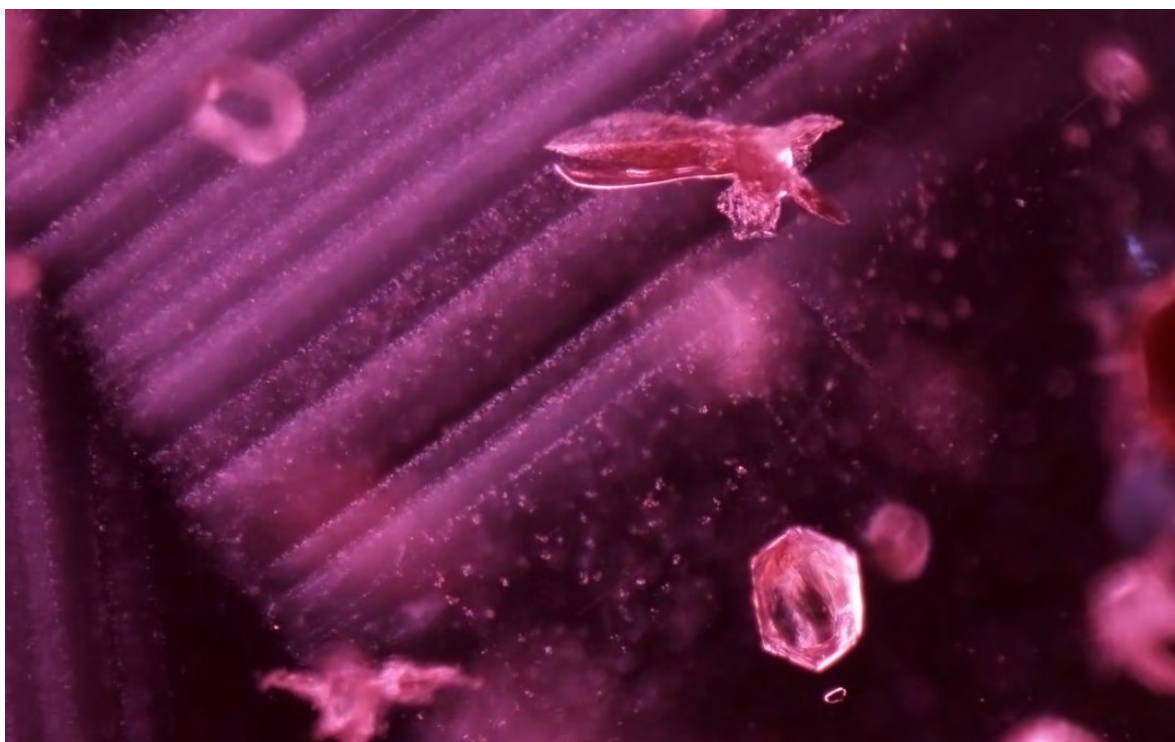
Figure 73: Bands of minute particles form a nice backdrop to hexagonal translucent mica crystals that show not all mica crystals are associated with frosty fringes in a Ruby from Montepuez. GIA reference sample number 100305163842, an F type sample obtained in Thailand in January 2013 in a parcel of “Bo Nam” rough. Darkfield illumination, magnified 70x. Photo: Jonathan Muiyal © GIA.
