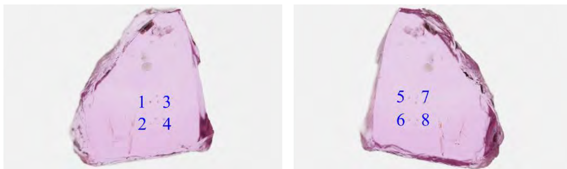
Figure 29: Two views of GIA reference sample 100305163907 (A2 type; see Annex C for a description of the classification system), seen after fabrication, showing the positions of the eight LA-ICP-MS spots. Photos (color calibrated): Sasithorn Engniwat © GIA.
