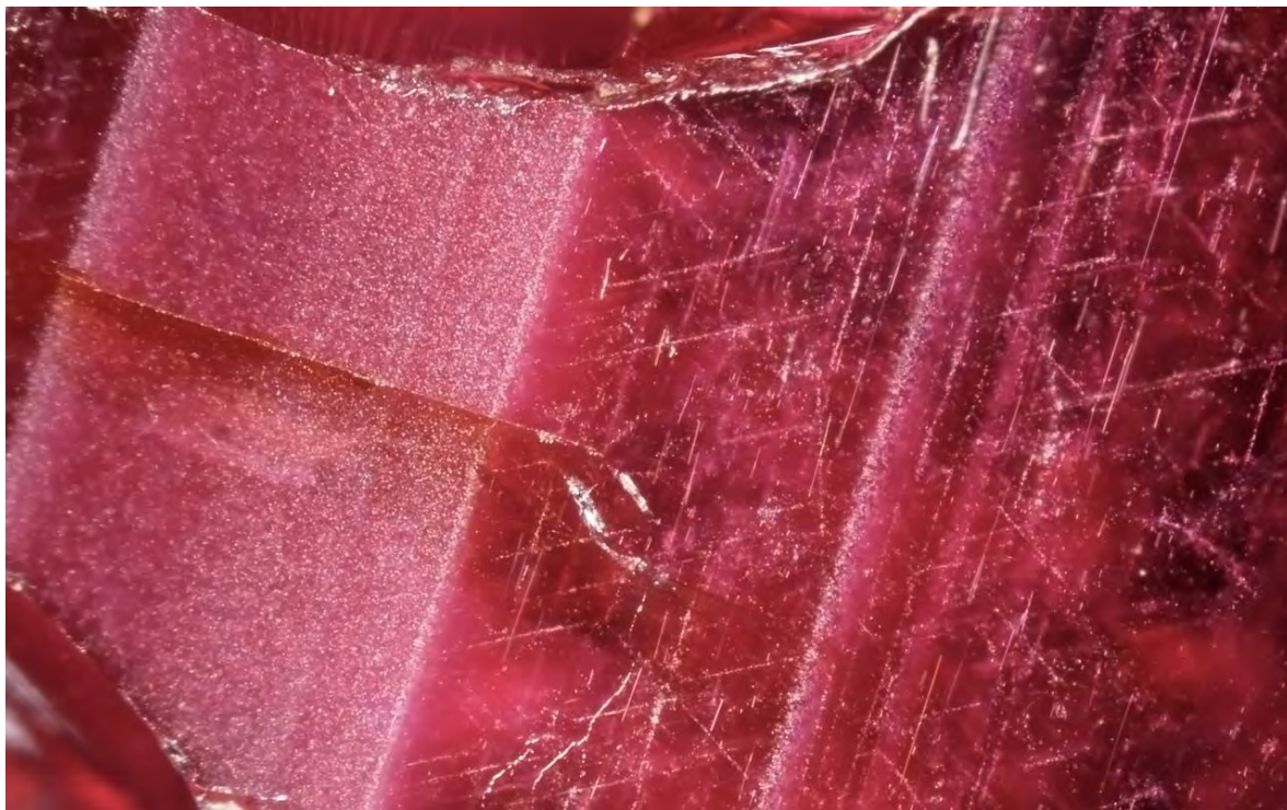
Figure 94: Broad and thin bands of minute whitish particles aligned at 60 degrees to each other resulting in very silky appearance to the stone. GIA reference sample 100305163946, a "B" type sample collected in the Namujo/Torro area in September 2012. Darkfield + fiber optic illumination, magnified 40x. Photo: Jonathan Muiyal © GIA.
