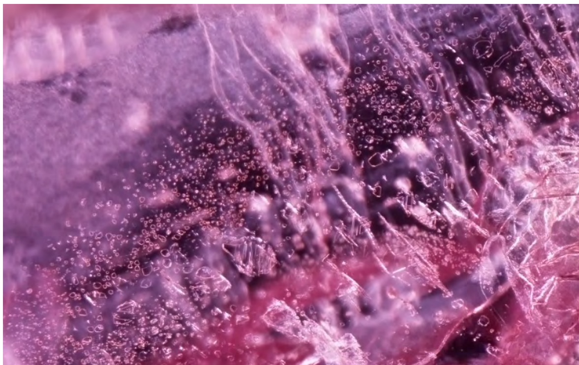
Figure 86: A plane of flat reflective particles (out of focus in the previous photo) associated with surface reaching fissures and negative crystals in a Ruby from Montepuez. GIA reference sample number 100305163938, an A type sample from the "Central" area collected on site in September 2012. Diffused + fiber optic illumination, magnified 80x. Photo: Jonathan Muyal © GIA.
