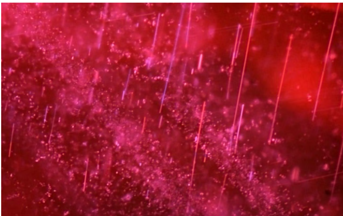
Figure 97: Detailed view of some bands of minute particles showing short and long thin needles within them aligned at 60 degrees to each other. GIA reference sample 100305164538, an “E” type sample (probably from the “Central” area) collected in Nampula in September 2009. Fiber optic illumination, magnified 80x. Photo: Jonathan Muyal © GIA.
