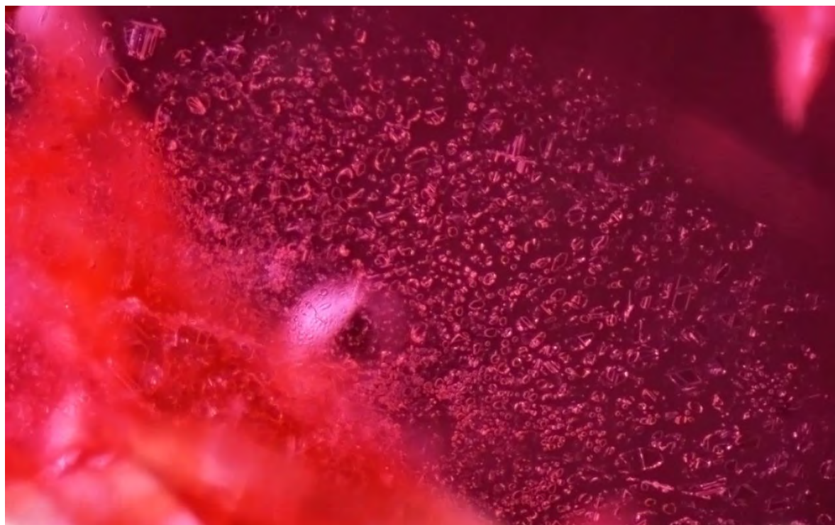
Figure 81: A plane composed of hundreds of small thin film like negative crystals forming a beautiful pattern in a Ruby from Montepuez. GIA reference sample number 100305163864, an F type sample obtained in Thailand in January 2013 in a parcel of “Bo Nam” rough. Transmitted + fiber optic illumination, magnified 100x. Photo: Jonathan Muiyal © GIA.
