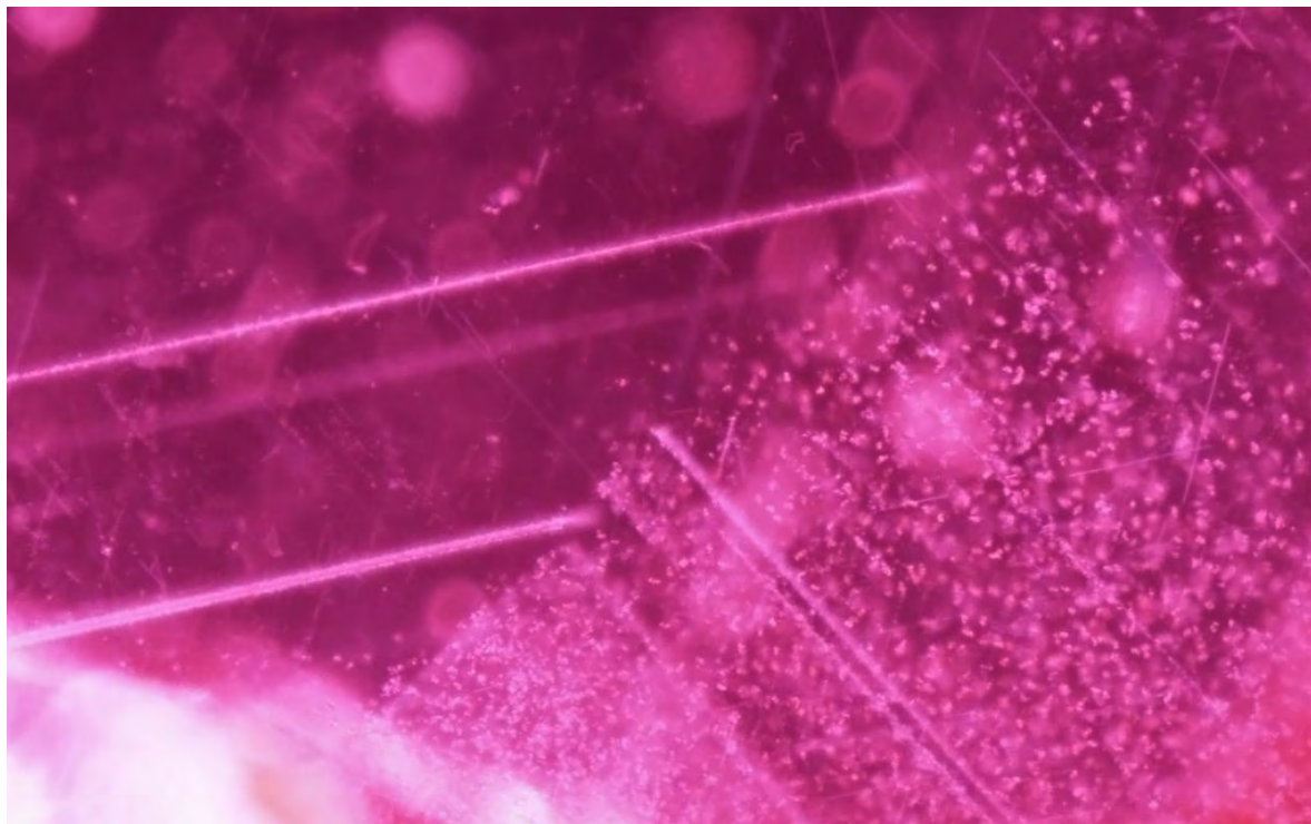
Figure 90: Bands of minute whitish particles forming part of a hexagonal pattern associated with long and short thin needles aligned at 60 degrees to each other. GIA reference sample 0668540102, an "E" type sample (probably from the "Central" area) collected in Nampula in September 2009. Darkfield + fiber optic illumination, magnified 40x. Photo: Jonathan Muyal © GIA.
