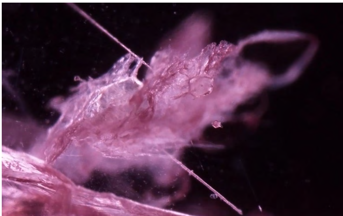
Figure 67: Mica crystals of varying sizes that are easy to recognize owing to their tabular, hexagonal, more translucent appearance and their characteristic associated frosty looking fringes. GIA reference sample number 0668531802, an E type sample (probably from the “Central” area) obtained in Mozambique in September 2009. Darkfield + fiber optic illumination, magnified 80x. Photo: Jonathan Muiyal © GIA.
