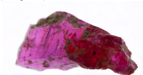
Figure 16: GIA reference sample 100305164174 (A1 type; see Annex C for a description of the classification system), weighing 1.530 carats seen before fabrication via transmitted light. The sample is clean on the left side and heavily included on the right side. Thus we decided to cut it in two pieces and use the left side for spectroscopy. This stone was collected on site in an exploration trench at "Central" on September 10 th 2012. Photo (color calibrated): Sasithorn Engniwat © GIA.
