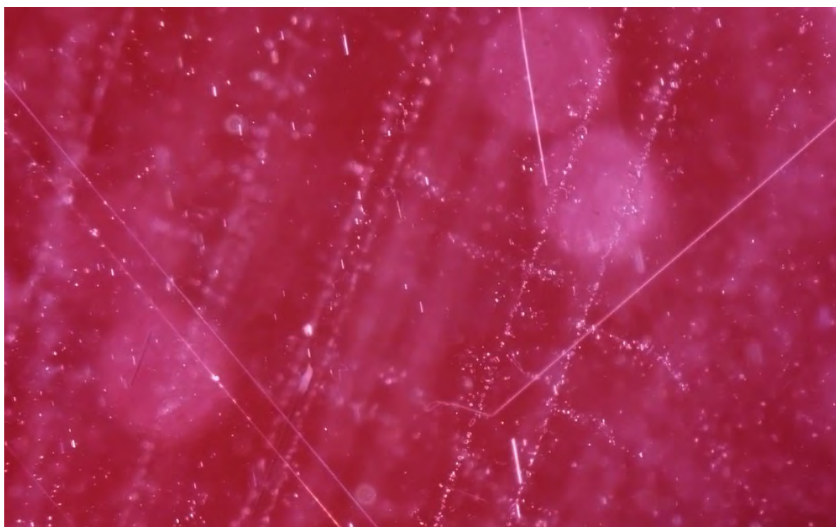
Figure 87: Parallel planes of minute and coarse whitish particles, crossing each other at 90 degrees, associated with long and short thin needles, crossing each other at 60 degrees, in a Ruby from Montepuez. GIA reference sample 0668532602, an "E" type sample (probably from the "Central" area) collected in Pemba in September 2009. Darkfield + fiber optic illumination, magnified 60x. Photo: Jonathan Muyal © GIA.
