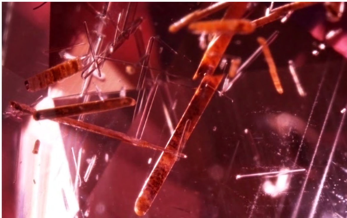
Figure 60: A group of long transparent acicular looking crystals (identified by Raman as amphibole using the RRuff database as a reference) associated with bands of minute particles seen in GIA reference sample number 100305164551, an F type sample obtained in Chanthaburi, Thailand in January 2013. Darkfield + fiber optic illumination, magnified 50x. Photo: Jonathan Muiyal © GIA.
