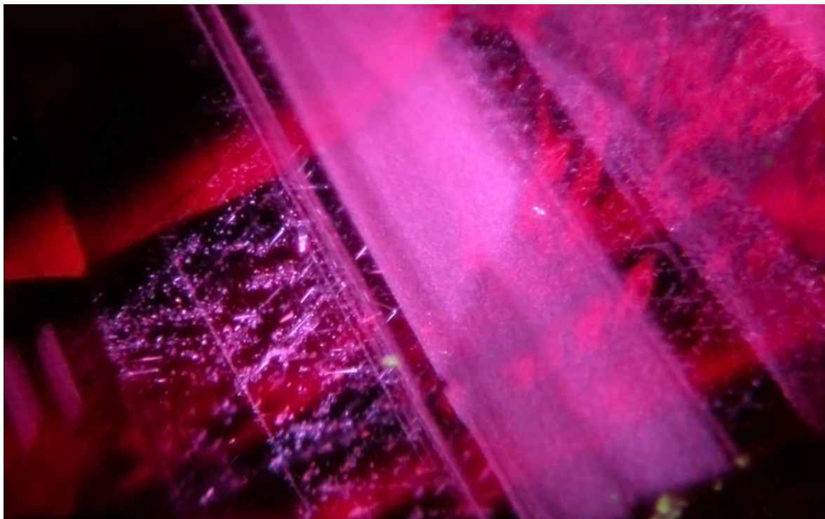
Figure 96: Broad bands of minute particles appearing as white clouds together with “arrow-head” needles aligned at 60 degrees to each other in a Ruby from Montepuez. Darkfield + fiber optic illumination, magnified 30x. Photo: Vincent Pardieu © GIA.
