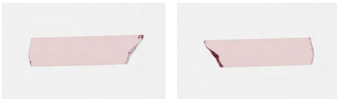
Figure 38: Two views of GIA reference sample 100305163945 (B2 type; see Annex C for a description of the classification system), weighing 0.066 carats seen after fabrications with windows cut in the direction perpendicular to the c-axis. In this orientation color is homogenous brownish pink. Photos (color calibrated): Sasithorn Engniwat © GIA.
