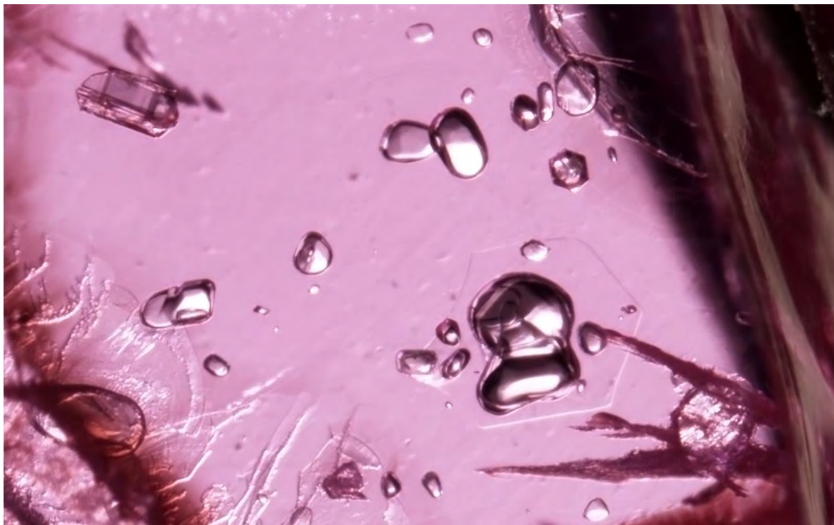
Figure 46: In this third photo of the same group of crystals, the importance of using different types of lighting environments while working with a microscope is clearly illustrated. Using transmitted light, the crystals still look transparent however several interesting growth features associated with the crystal inclusions now become more apparent. GIA reference sample number 100305163938 from the “Central” area. Brightfield + fiber optic illumination, magnified 40x. Photo: Jonathan Muiyal © GIA.
