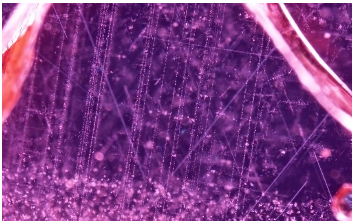
Figure 89: A very busy inclusion scene showing bands of minute whitish particles arranged parallel, or 90 degrees to each other, associated with long and short rutile like needles aligned at 60 degrees to each other. GIA reference sample 0668538702, an "E" type sample (probably from the "Central" area) collected in Nampula in September 2009. Darkfield + fiber optic illumination, magnified 40x. Photo: Jonathan Muyal © GIA.
