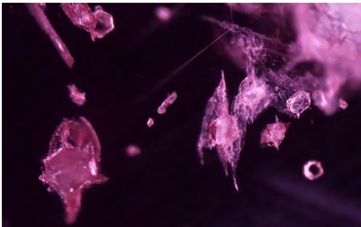
Figure 65: A group of hexagonal, translucent mica crystals associated with their characteristic frothy looking fringes. GIA reference sample number 100305163853, an F type sample obtained in Thailand in January 2013 in a parcel of “Bo Nam” rough. Darkfield + fiber optic illumination, magnified 70x. Photo: Jonathan Muiyal © GIA.
