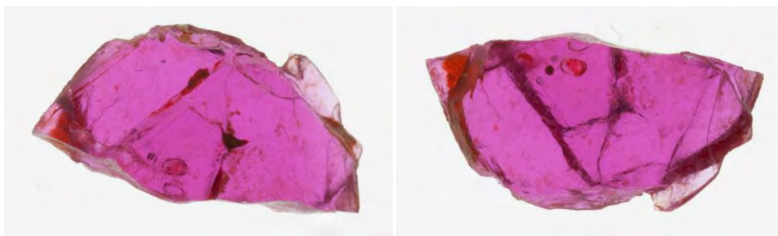
Figure 31: Two views of GIA reference sample 100305163897 (A2 type; see Annex C for a description of the classification system), weighing 0.121 carat seen before fabrication. The color, via transmitted light is deep purplish pink with a homogeneous color distribution. Photos (color calibrated): Sasithorn Engniwat © GIA.
