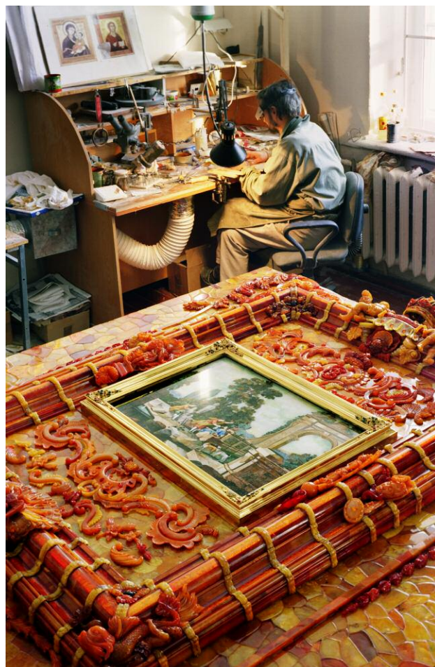
Figure 8. A craftsman in the Tsarskoye Selo Amber Workshop completing a carving for the mosaic “Touch and Smell” from slices of jasper, malachite, quartz, chalcedony, and nephrite. Photo courtesy of Tsarskoye Selo Amber Workshop.
