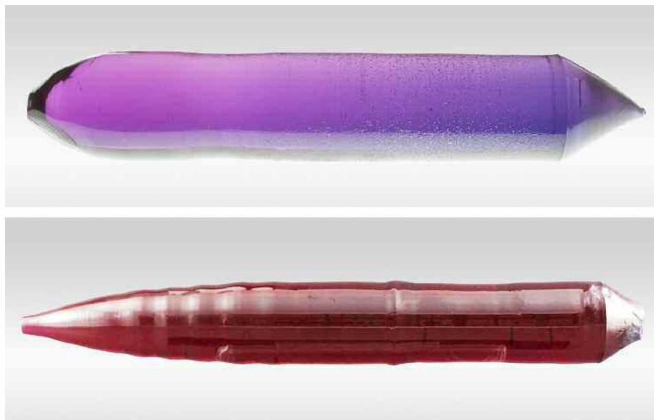
Figure 2. Crystal boules grown by Scientific Materials for multi-doped corundum standards: sample 02-1032 (top) and sample 07-0687 (bottom). Both crystals were doped with Mg, Ti, V, Cr, and Ga in different amounts; only 02-1032 was successfully doped with Fe. Crystal 02-1032 is 40 mm in diameter by 150 mm in length at diameter, and crystal 07-0687 is 30 mm in diameter by 150 mm in length at diameter. Photos courtesy of Scientific Materials.
