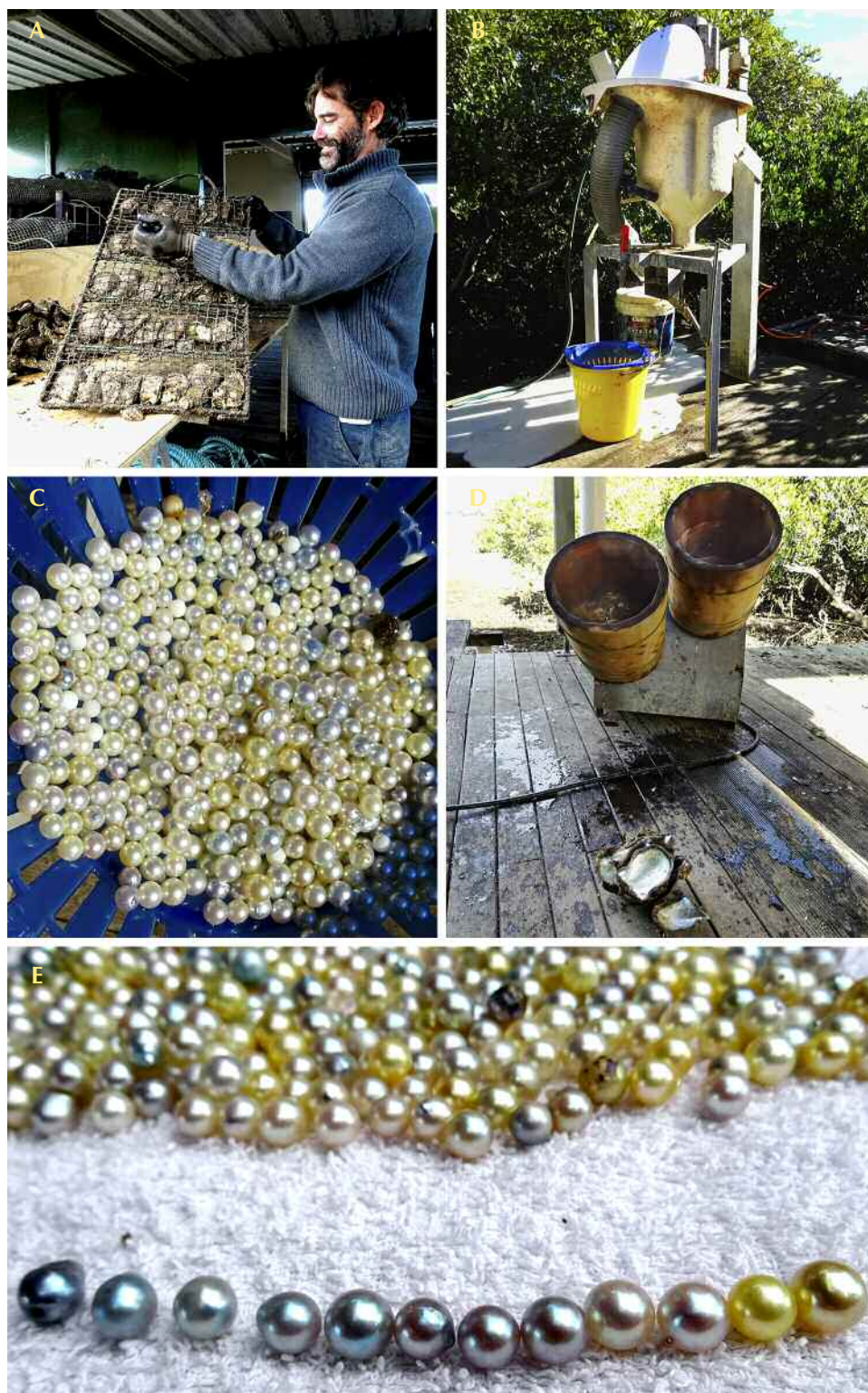
Figure 5. The steps involved in the process of harvesting Australian akoya pearls. A: Bivalves are removed from their cages. B: The separator cleans the pearls from the tissues. C: Separated pearls are collected by opening a valve at the bottom of the machine. D: Wooden revolving drums are used to wash the pearls in a saltwater solution. E: A selection of the day's harvest with the range of colors displayed at the front. Photos by Laura Otter.
