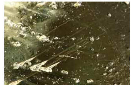
Figure 10. Etch tubes extended from surface etch pits and ended at the twinning plane. Field of view approximately 2.30 mm.
