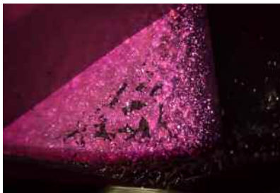
Figure 13. Reflective silk inclusions in the natural sapphire seed are visible behind a coarse flux fingerprint in the synthetic ruby overgrowth, which was cut through during the fashioning process. Field of view 3.57 mm.
