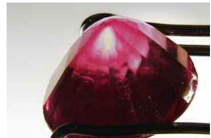
Figure 14. A portion of the near-colorless corundum seed is revealed in an area where the synthetic ruby overgrowth was cut away during fashioning. Field of view 10.85 mm.
