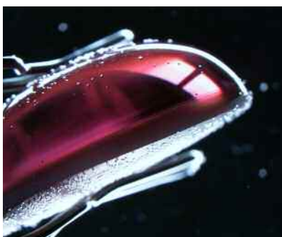
Figure 2. A side view of the cabochon, immersed in water, showing the localized inclusions near the base. Field of view 1.6 cm.
