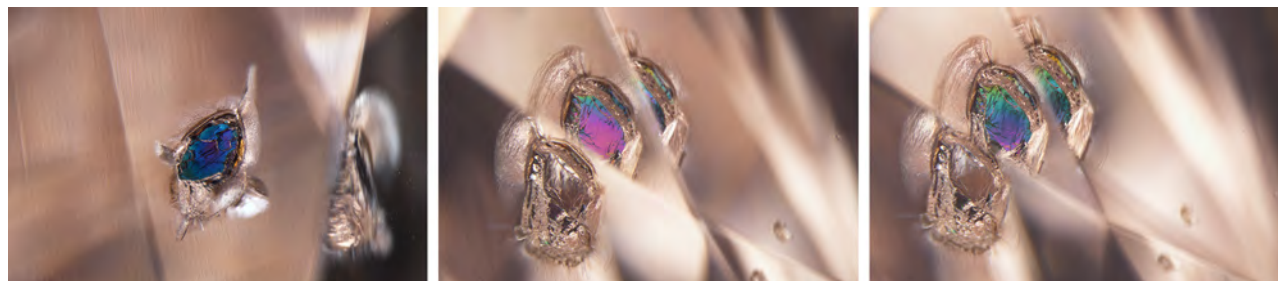
Figure 5. The changing iridescent colors of a ferropericlase inclusion are revealed through different facets of the host diamond. Photomicrographs by Evan M. Smith; field of view 1.99 mm.
