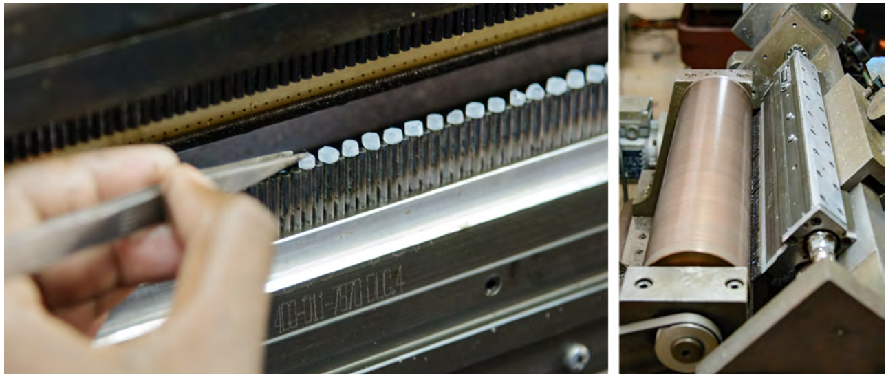
Figure 17. Numerous calibrated preforms are placed on a computerized faceting machine for final calibration, faceting, and polishing at RMC. Photos by Andrew Lucas, courtesy of RMC.
