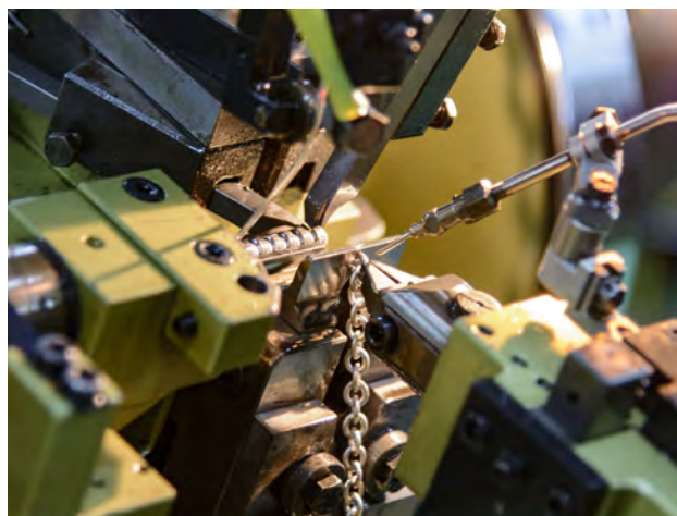
Figure 36. An assortment of chain-making machines in Derewala's factory are capable of creating numerous styles in silver and various gold karat alloys. Photo by Andrew Lucas, courtesy of Derewala.
