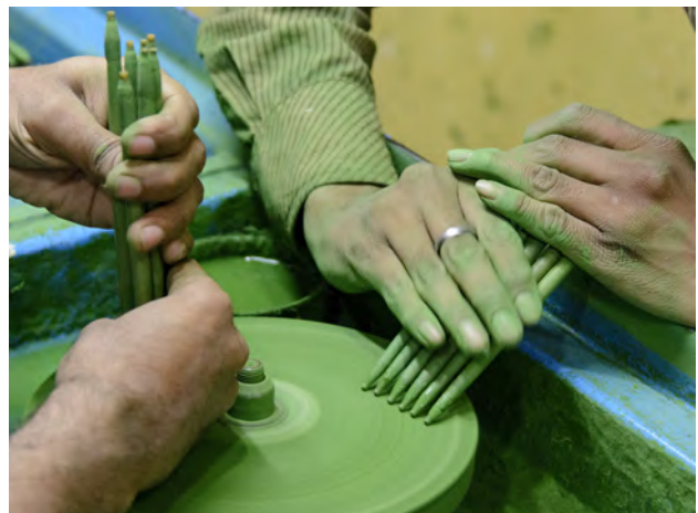
Figure 18. Faceting colored gemstones by hand is still highly effective, even when a million stones per month are required. Photo by Andrew Lucas, courtesy of RMC.
