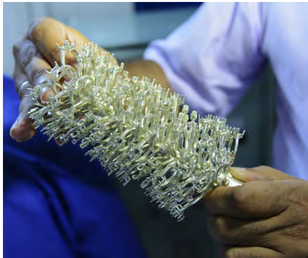
Figure 39. By investing in sophisticated vacuum casting equipment and incorporating strict casting procedures, Pink City can produce high-quality castings, a crucial first step in quality control. Photo by Andrew Lucas, courtesy of Pink City Jewel House.
