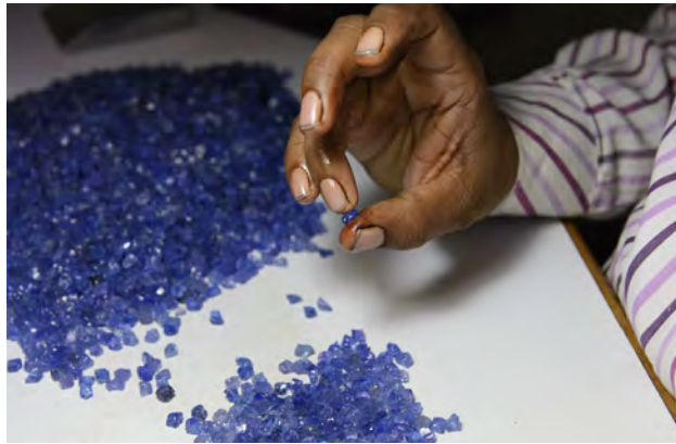
Figure 15. While the facet-grade tanzanites available to MeM Gems are under one gram in size, the company still has an extensive rough sorting system for shape, color, and clarity that provides consistent quality ranges for cut stones. Photo by Andrew Lucas, courtesy of MeM Gems.
