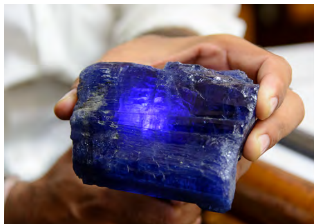
Figure 12. With its expertise in evaluating tanzanite rough, AG Gems can buy larger cabochon-grade pieces and cut transparent areas for large faceted stones. Part of evaluating the rough is observing its pleochroism and finding the more valuable intense bluish and purple color directions. Photos by Andrew Lucas, courtesy of AG Gems.
