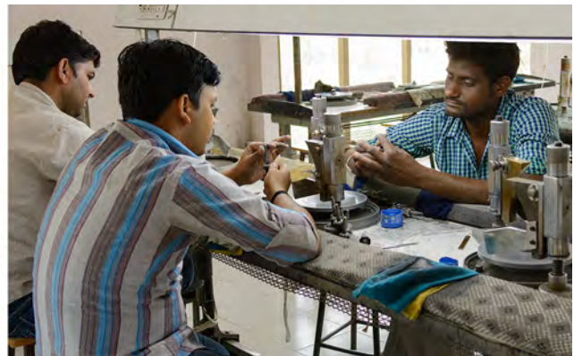
Figure 20. Sambhav's preformers and faceters are shown cutting morganite and fire opal. Photos by Andrew Lucas, courtesy of Sambhav Jewels.
