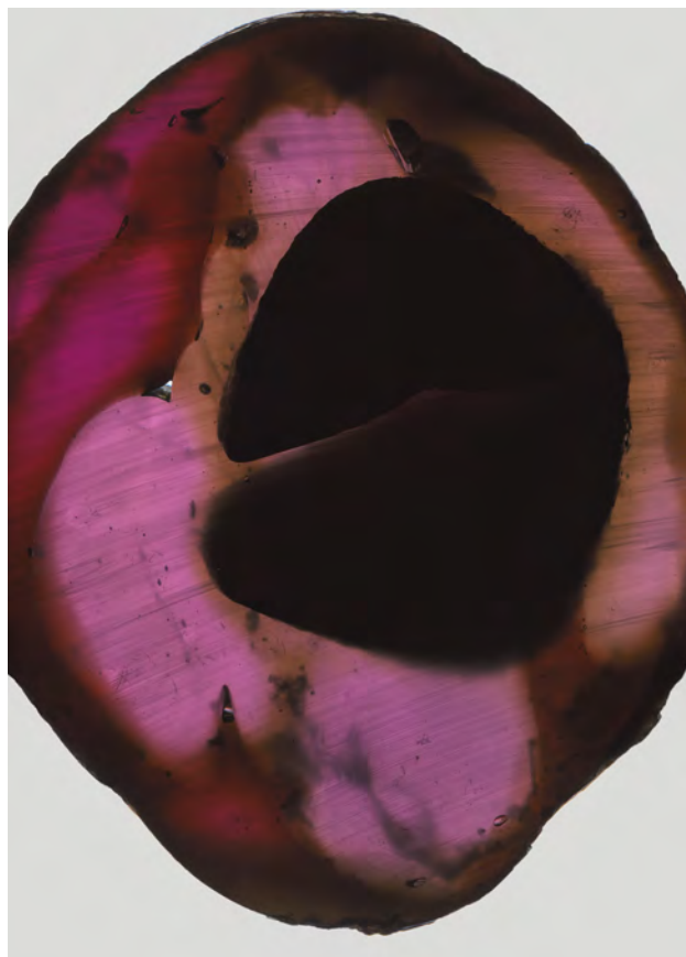
Figure 13. A transparency scan of an imitation boulder section; the black region is the metal insert. Color changes in different areas of the boulder suggest a multiple-step preparation involving various resin batches. The resins may have been worked in a semi-fluid or solid but malleable form, because some lack of adhesion—and the creation of voids—is noticeable. Photo by Emanuele Costa.
