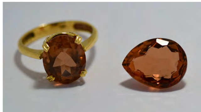
Figure 15. These glass imitations of Zultanite are shown in fluorescent (left) and incandescent light (right). The color-change effect is apparent when switching between the two illumination types. Photos by Xiaoyan Yu.
