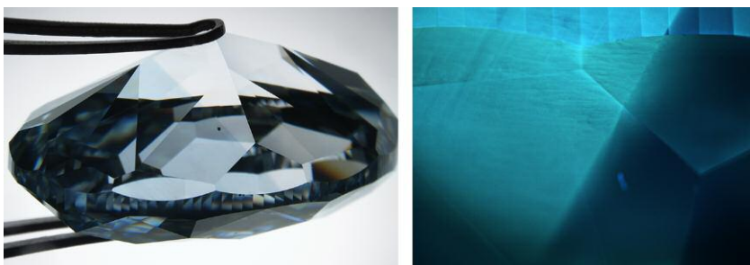
Figure 7. Color zonation (left) becomes more noticeable when viewed through the pavilion. The stronger blue-colored region corresponds with bright greenish blue fluorescence in the DiamondView (right, field of view 5.8 mm). Note that the DiamondView image is taken from the opposite side of the diamond.
