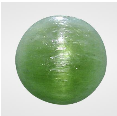
Figure 13. This 1.42 ct translucent variegated green bead displays a distinct chatoyant band on the darker green side (left). No chatoyancy was observed on the lighter green side (right).
