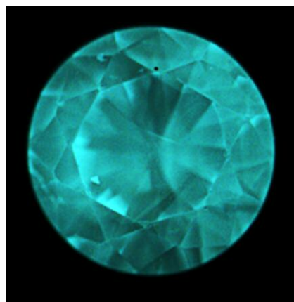
Figure 9. This diamond shows characteristic growth patterns of HPHT-grown material.
