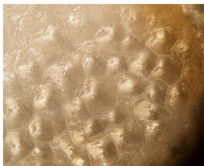
Figure 21. Left: A 3.09 ct cabochon showed various surface structures consisting of a non-directional patchwork of cells near the center to a broad mottled appearance in the outer area, together with natural brownish layers of shell formation. Right: Higher magnification of another cabochon's surface revealed a distinct patchwork structure. Both samples displayed a whitish sheen on the surface when illuminated with a fiber-optic light. Fields of view 11.90 mm (left) and 5.24 mm (right).
