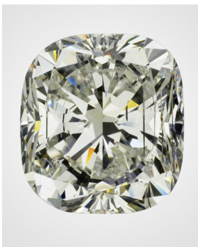
Figure 29. This 15.32 ct cushion modified brilliant, with grades equivalent to H color and I_1 clarity, is the largest HPHT synthetic diamond graded by GIA.
