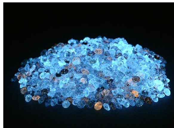
Figure 10. These HPHT-grown synthetic diamond melee, from the parcel of 1,102 specimens, display strong phosphorescence following exposure to short-wave UV radiation.
