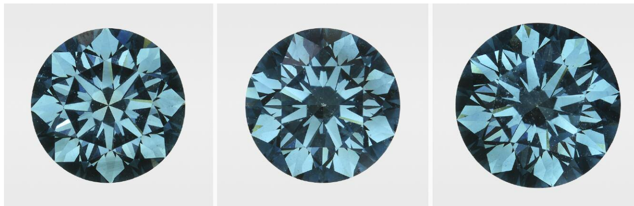
Figure 24. These 1.12 ct, 1.14 ct, and 1.34 ct laboratory-irradiated CVD synthetic diamonds all have similar appearance, with color grades equivalent to Fancy Deep green-blue.
