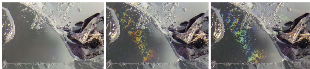
Figure 2. The surface of the aquamarine crystal contains a hidden iridescence that is only visible when the light source is at certain angles relative to the surface of the stone. The angle of the oblique fiber-optic illumination in the photo on the left does not make the iridescence visible. As this light is swept across the surface, changing the angle of illumination, colorful iridescent colors appear (center). The appearance of the phenomenon alters along with the angle of illumination (right). The large dark area in the right portion of each image is a reflective void. Photomicrographs by Nathan Renfro; field of view 4.8 mm.
