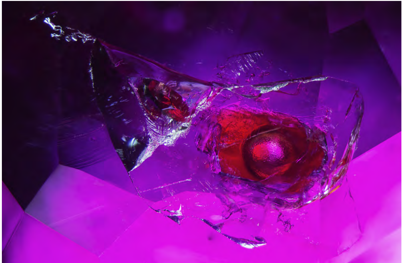
Figure 9. The red color of the oil within the cavity of a ruby displays a remarkable contrast with the bodycolor of the gem. Unlike the flattened bubbles regularly encountered, a rounded bubble attests to the size of the cavity containing the oil. Photomicrograph by E. Billie Hughes; field of view approximately 2.5 mm.
