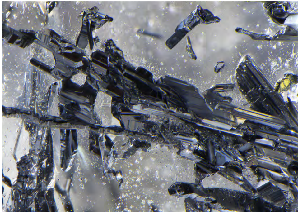
Figure 7. Displaying an orthorhombic morphology, these inclusions were identified as cosalite. Photomicrograph by Nathan Renfro; field of view 4.11 mm.
