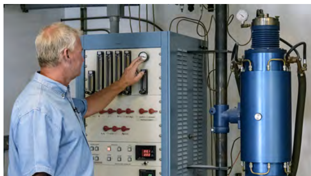
Figure 19. Chris Cooney of Gem Mountain Sapphire Mine operates the electrical furnace used to heat sapphires. The metallic blue cylinder to the right of the control panel houses the sapphire-containing crucibles. Photo by Andrew Lucas.
