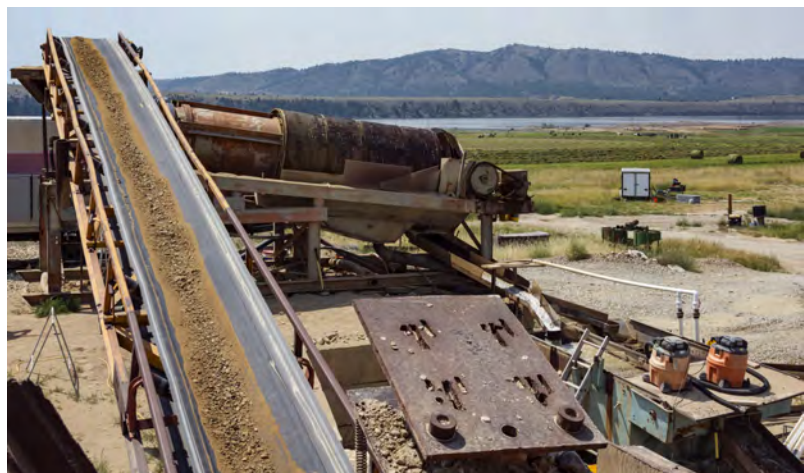
Figure 8. At Eldorado Bar, the washing plant is set up on the gravel bar. Sapphire-bearing gravels are fed through an oversized screen and a trommel, then sorted by a set of jigs and a sluice box for gold and very small sapphire recovery. The operation lies next to the river and some beautiful grassland. Photo by Andrew Lucas.
