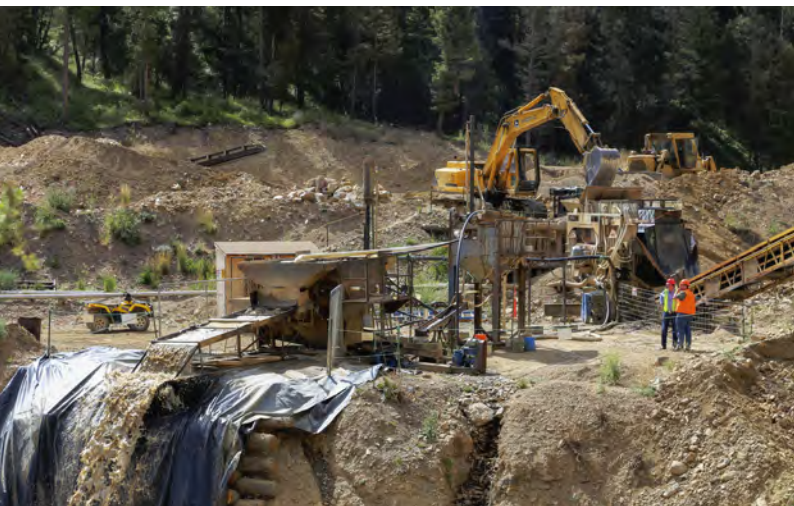
Figure 15. Both sapphire and gold are recovered at Potentate's washing plant at Eureka Gulch. The washing plant has a feeder, an oversized screen, multiple conveyor belts, and two sets of jigs, along with a sluice box used mainly to recover gold and very small sapphires. Photo by Andrew Lucas.
