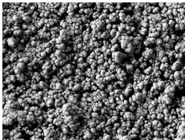
Figure 6. SEM image of the heterogeneous nanostructure of a common gem opal from the Cuitzeo area in Michoacán. The spheres are too small, irregularly sized, and disorganized to exhibit play-of-color.
