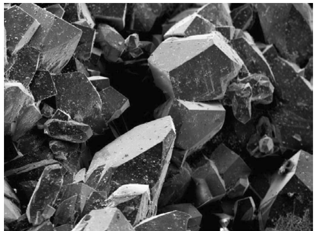
Figure 22. SEM imaging shows the small, well-shaped quartz crystals within the cavities. The crystal in the lower middle clearly displays the classic "flute" termination typical of quartz. Image by Emanuele Costa; field of view 1 mm.
