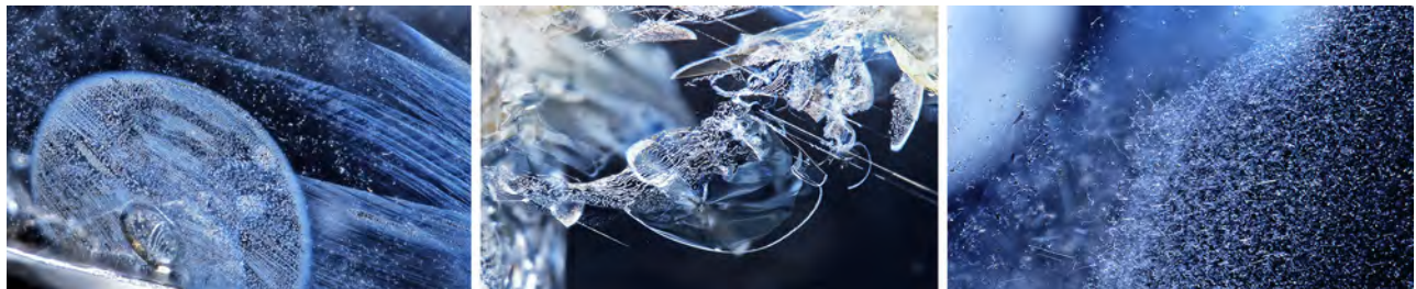
Figure 3. Left: An unidentified crystal surrounded by a fingerprint. Many particles and fine wispy fingerprints can be seen throughout the stone in darkfield lighting. Center: Intersection tubules associated with different types of fingerprints, shown here in fiber-optic lighting, were always found in the twinning planes of the Ethiopian sapphires. Right: Bands of particles seen with fiber-optic lighting. Photomicrographs by Victoria Raynaud; fields of view 1.20 mm (left), 3.60 mm (center), and 1.44 mm (right).
