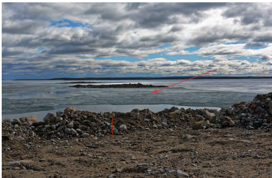
Figure 12. The A21 kimberlite pipe lies beneath the still-frozen waters of Lac de Gras. Its location is indicated by the red arrow. The future water retention dike will extend from the land at both edges of the photo to the nearer of the two islands. Once the dike is constructed, open-pit mining of the pipe can begin. Photo by James Shigley.
