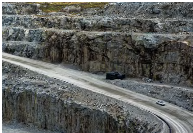
Figure 11. This view of the A418 open pit shows several of the mining benches as well as the access road that originally used to remove kimberlite ore from the pit and is now used for the underground workings. The pickup truck gives some indication of the benches' height. Photo by James Shigley.
