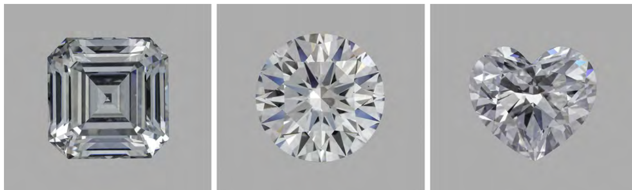
Figure 22. The emerald cut on the left is the largest colorless HPHT synthetic diamond ever reported (10.02 ct, E color). The other two, a 5.06 ct round and a 5.05 heart, both had D color.
