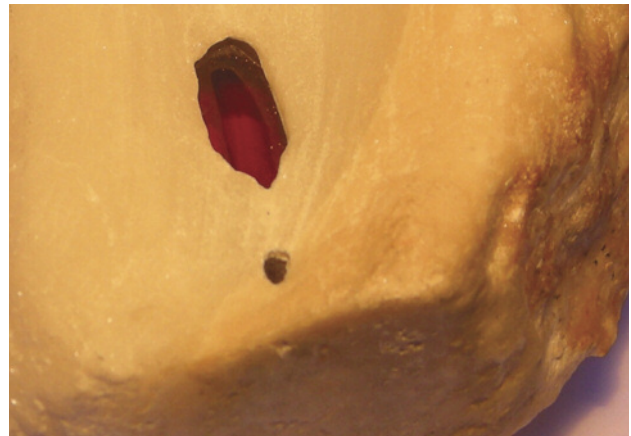
Figure 14. The synthetic ruby was embedded in a calcite matrix, seen here under incandescent light. Photo by Nazar Ahmed, Dubai Central Laboratory.
