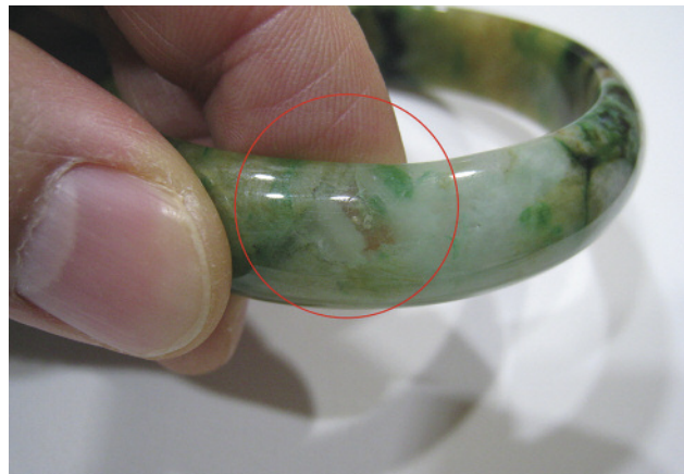
Figure 2. Microscopic examination of the suspect area revealed natural inclusions and a crystalline form. Neither would be found in an impregnated specimen. Photo courtesy of Lai Tai-An Gem Lab.
