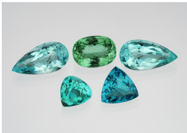
Figure 8. Cuprian liddicoatite and cuprian elbaite, species determined by LA-ICP-MS. Top row, left and right: 3.80 ct and 4.14 ct greenish blue cuprian liddicoatite, courtesy of Hubert Gesser at Hubert Inc. Top row, center: 3.16 ct bluish green cuprian liddicoatite, courtesy of John R. Evans. Bottom row from left to right: 2.59 ct and 2.12 ct greenish blue cuprian elbaite, courtesy of the GIA Museum. Photo by Orasa Weldon.
