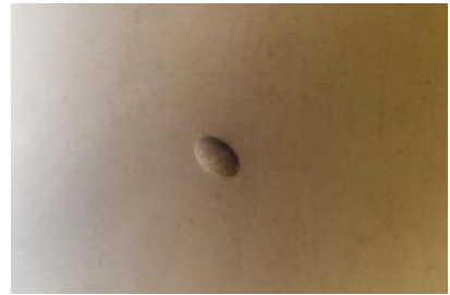
Figure 7. An elongated gas bubble seen below the surface of the white bangle. Field of view 3.57 mm.
