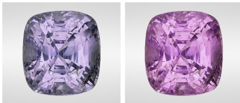
Figure 15. This 5.68 ct cushion mixed-cut sapphire showed a strong color change from grayish violet in fluorescent light to purple-pink in incandescent light.
