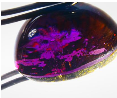
Figure 3. Viewed from the side, the assemblage was obvious. Trapped bubbles in the cemented plane can also be seen.
