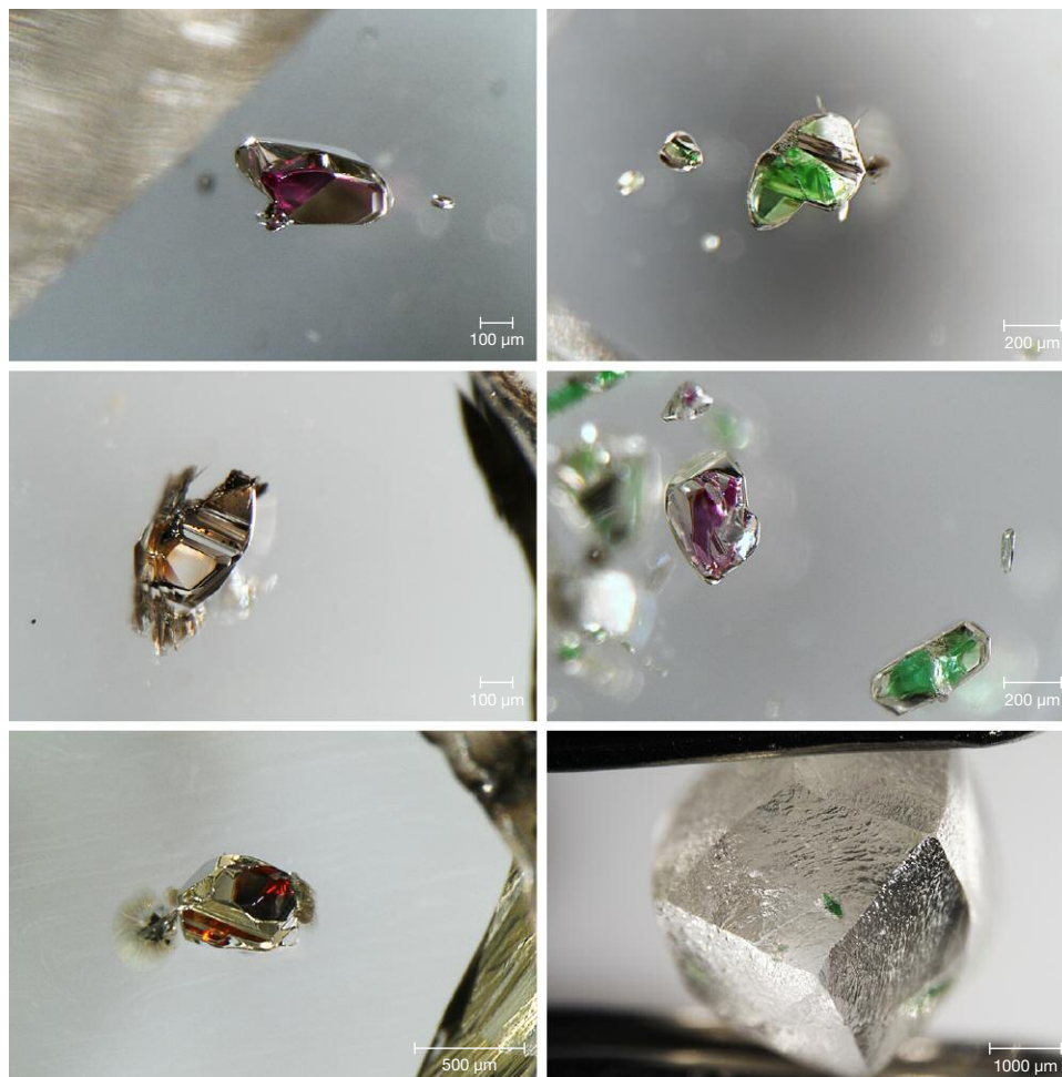
Figure 1. Orange-red-purple garnet and green clinopyroxene minerals included in diamond can be broken out, dissolved, and analyzed for their samarium-neodymium (Sm-Nd) and rubidium-strontium (Rb-Sr) isotopes to yield ages for diamond formation. Minerals such as these provided the first-ever ages for diamonds, proving that diamonds are forever and much, much older than their host kimberlite (Richardson et al., 1984). Photos by Karen Smit.
