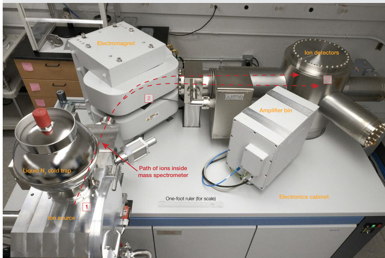
Figure C-1. The Thermo Scientific Triton Plus mass spectrometer used at the Carnegie Institution for Science. Photo by Steven Shirey.
