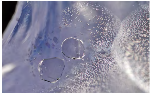
Figure 13. These two large primary fluid inclusions containing a black solid phase are associated with fingerprints that have a variable orientation. The photo was taken along the c-axis in darkfield illumination. Photomicrograph by Victoria Raynaud; field of view 1.07 mm.
