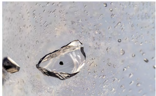
Figure 14. Left: A large fluid inclusion containing a CO 2 gas bubble and a marcasite crystal. The primary inclusion is surrounded by smaller inclusions that make up a healed fissure. Right: When the sample was gently heated, the gas bubble disappeared as the gas and liquid homogenized. The sample is illuminated using diffused backlighting. Photomicrographs by Victoria Raynaud; field of view 1.20 mm.
