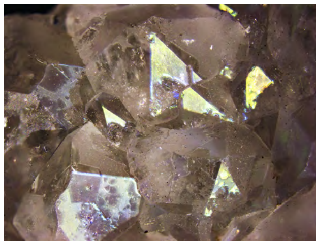
Figure 1. Iridescence is clearly visible on the minor z face of this iris quartz from Jalgaon, India. Photomicrograph by Peter J. Heaney; field of view 4.5 mm.
